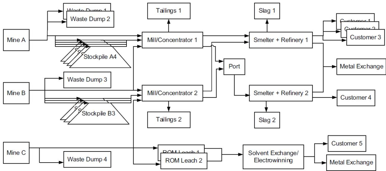
**Figure 1** An example of a mining complex with multiple mines, stockpiles, processing streams, and sales options (Goodfellow, 2014)
