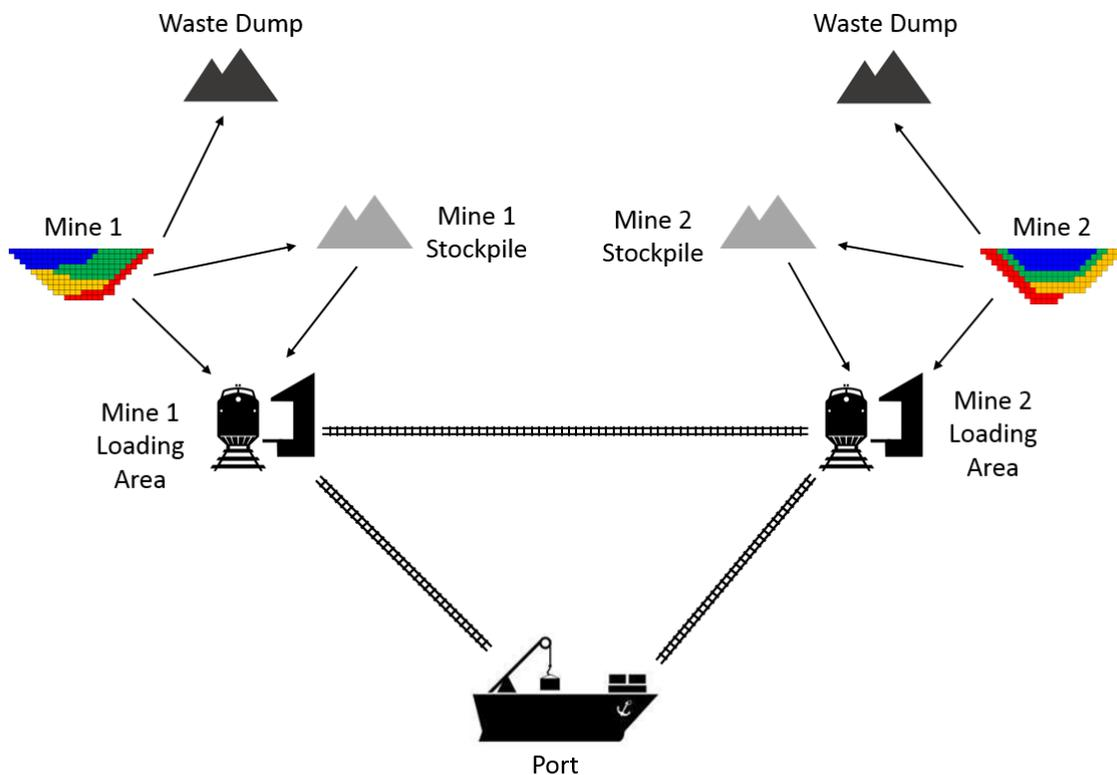
**Figure 17** Components and layout of the mining complex
