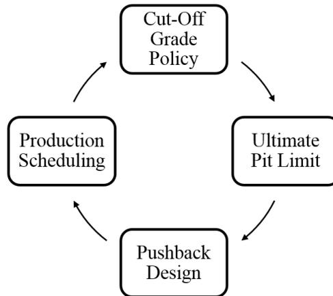
**Figure 2** Traditional production scheduling procedure
