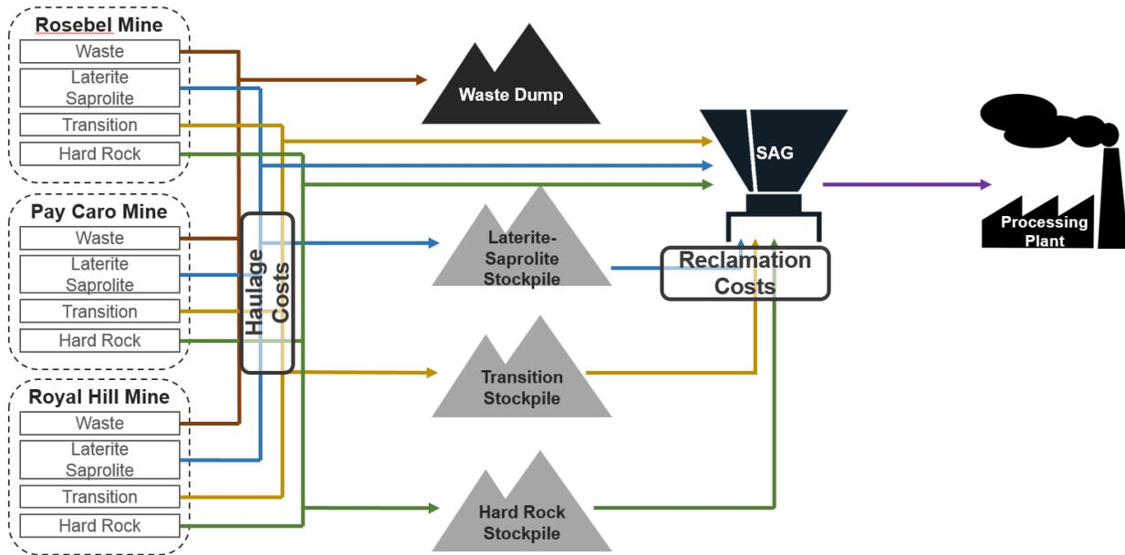
**Figure 3** Material flow diagram at the gold mining complex considered in this case study
