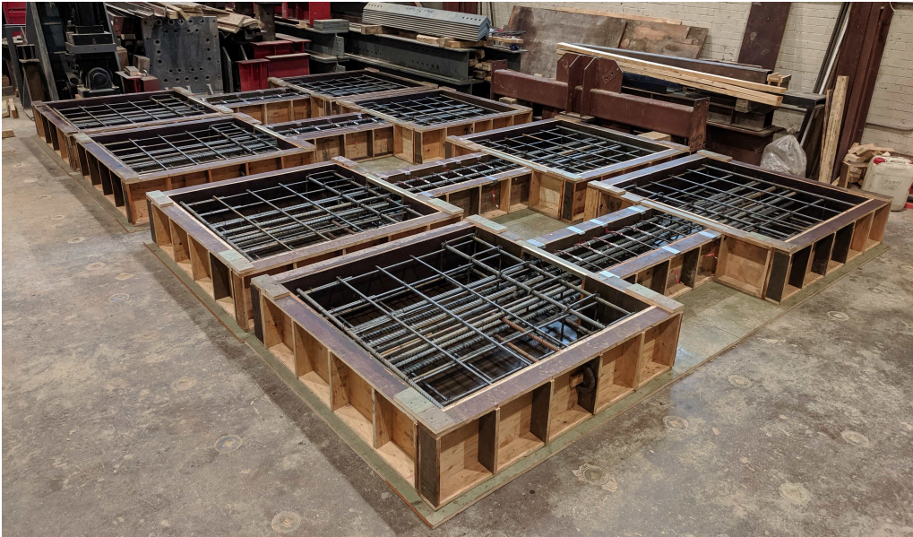
Figure 3.12: Specimens M1 and M2 in formwork before casting
