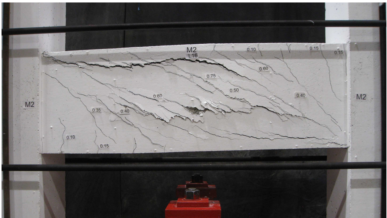
Figure 4.16: Shear failure of specimen M2
