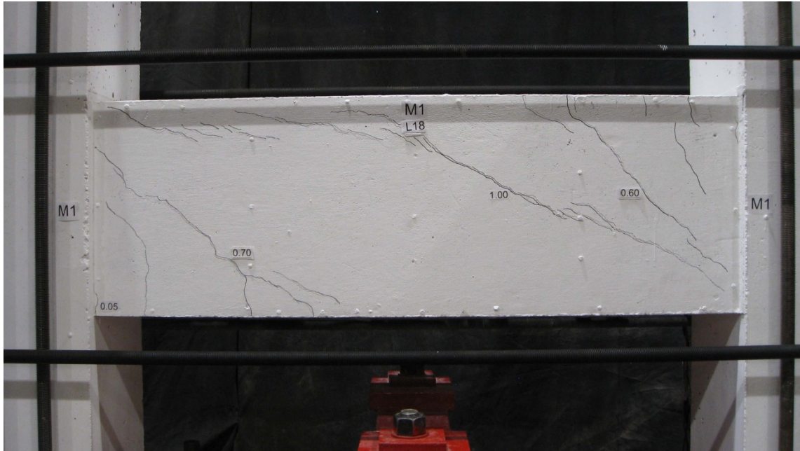
Figure 4.8: Crack pattern and widths at peak shear of 339 kN for specimen M1
