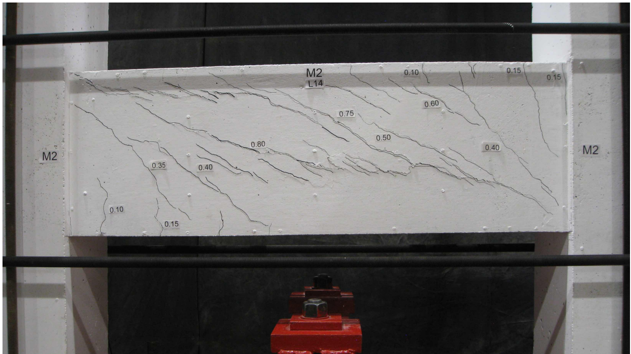
Figure 4.16: Shear failure of specimen M2
