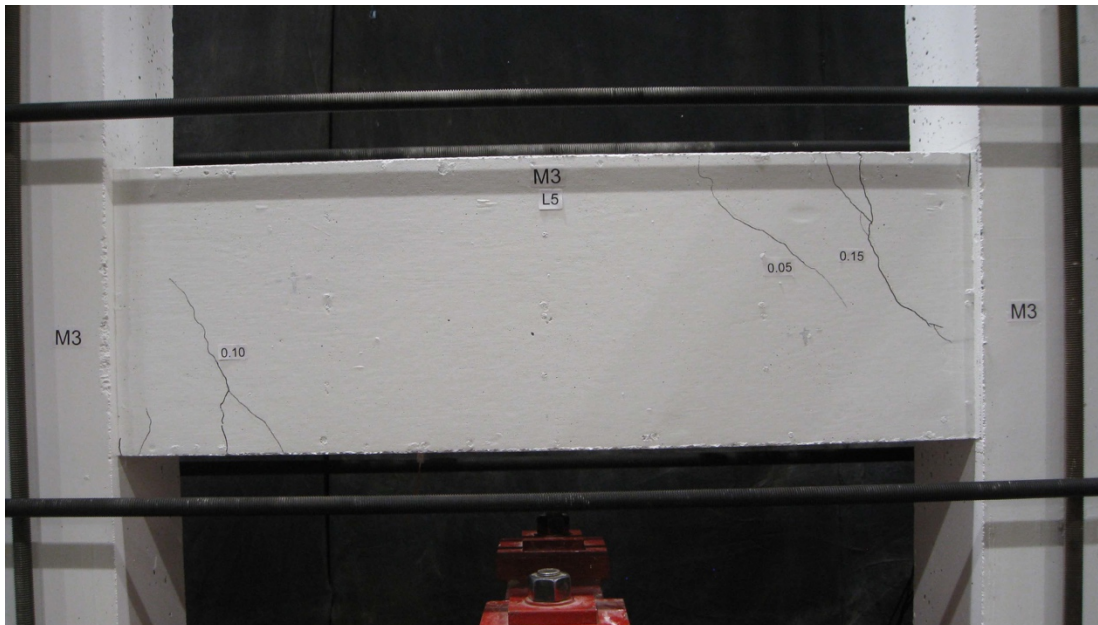
Figure 4.33: Crack pattern and widths at a shear of 242 kN for specimen M3
