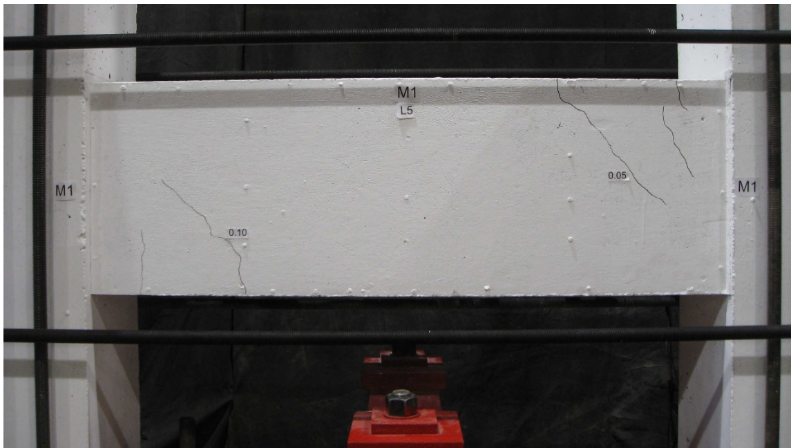
Figure 4.7: Crack pattern and widths at a shear of 225 kN for specimen M1
