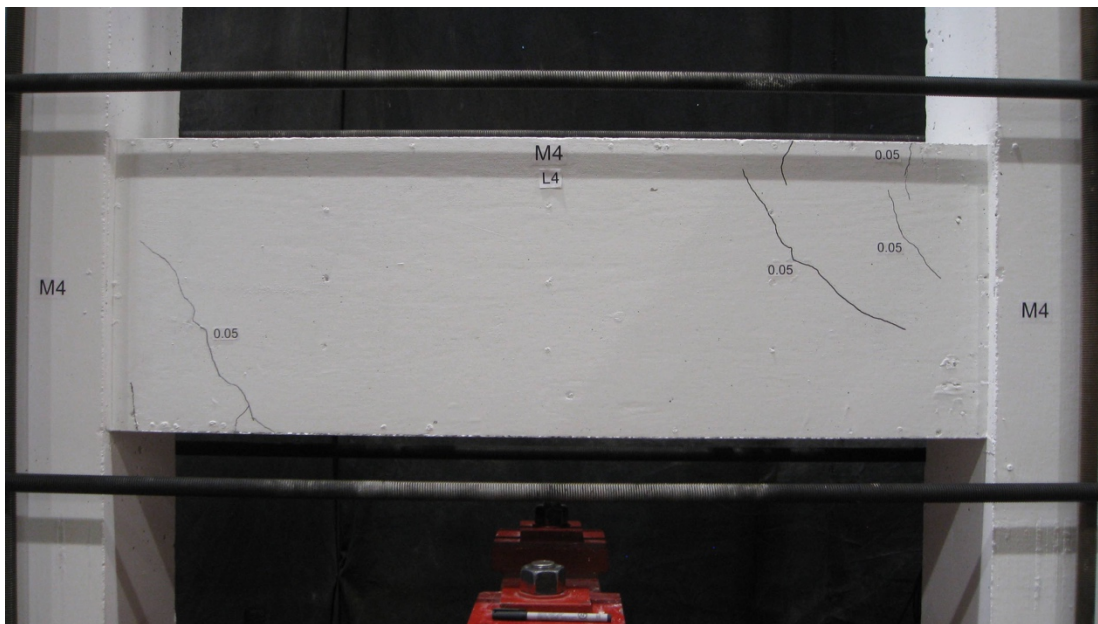
Figure 4.46: Crack pattern and widths at a shear of 226 kN for specimen M4
