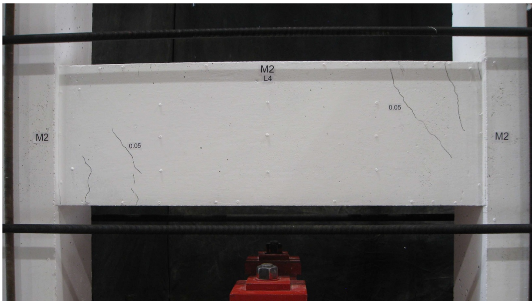
Figure 4.20: Crack pattern and widths at a shear of 226 kN for specimen M2
