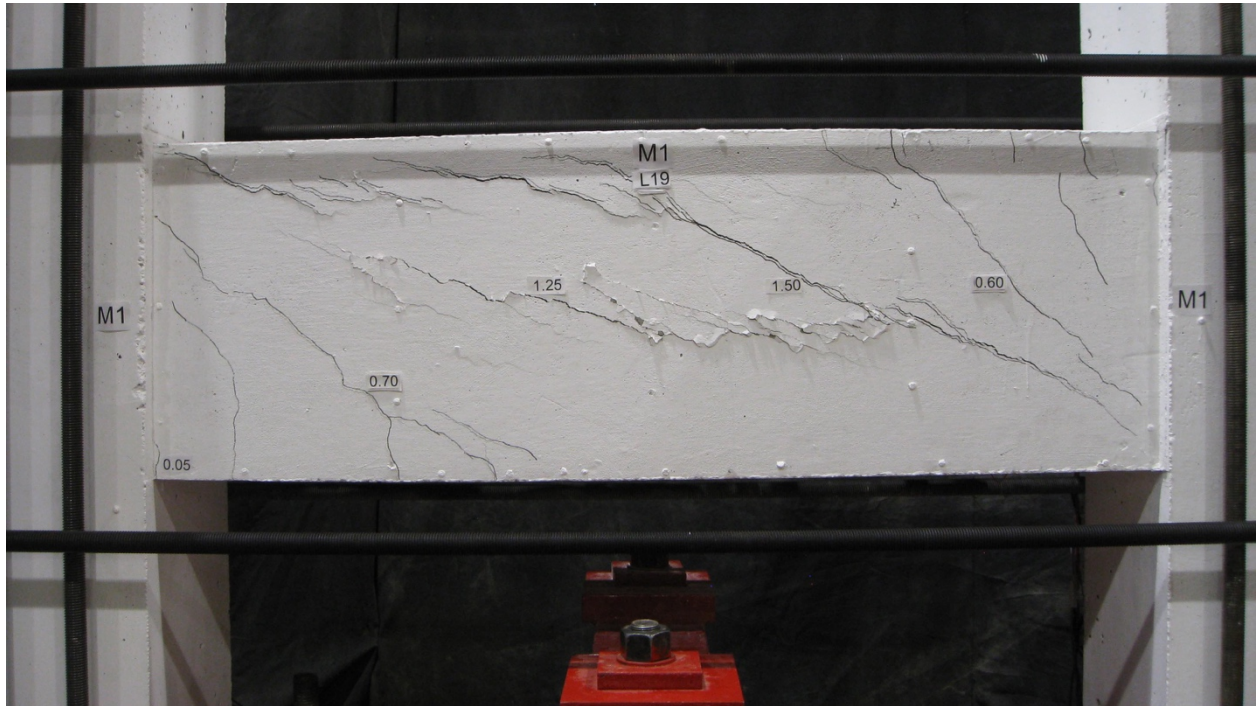
Figure 4.3: Shear failure of specimen M1
