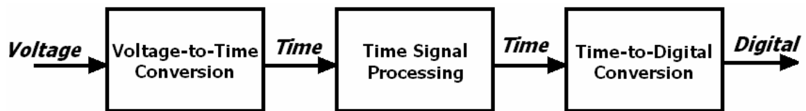
Figure 3.2: Block diagram of the analog-to-digital conversion process via time-mode signal processing.
