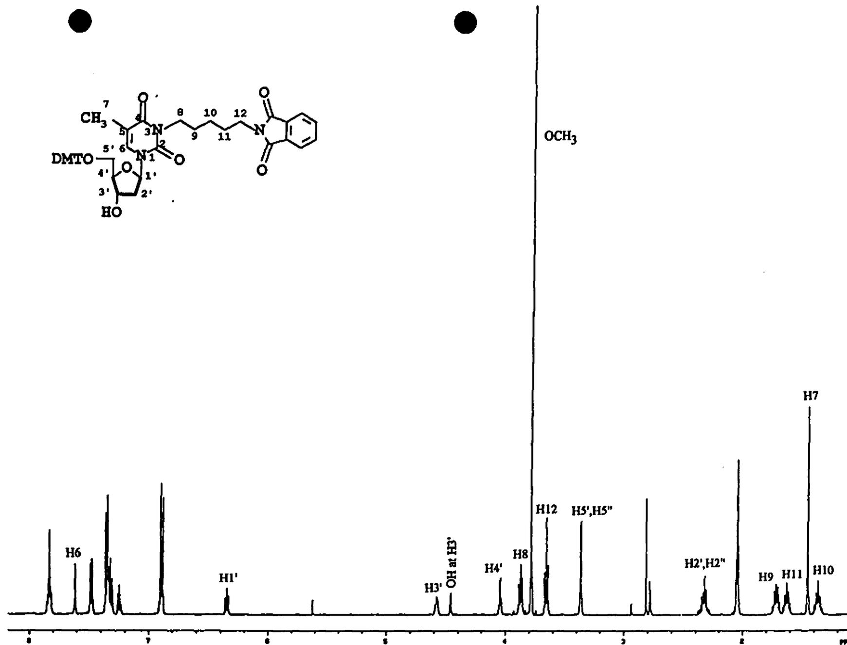
Figure 2.2 The 500 MHz <sup>1</sup>H-NMR spectrum of 7 in acetone-d<sub>6</sub> (chemical shifts are given in table 1).
