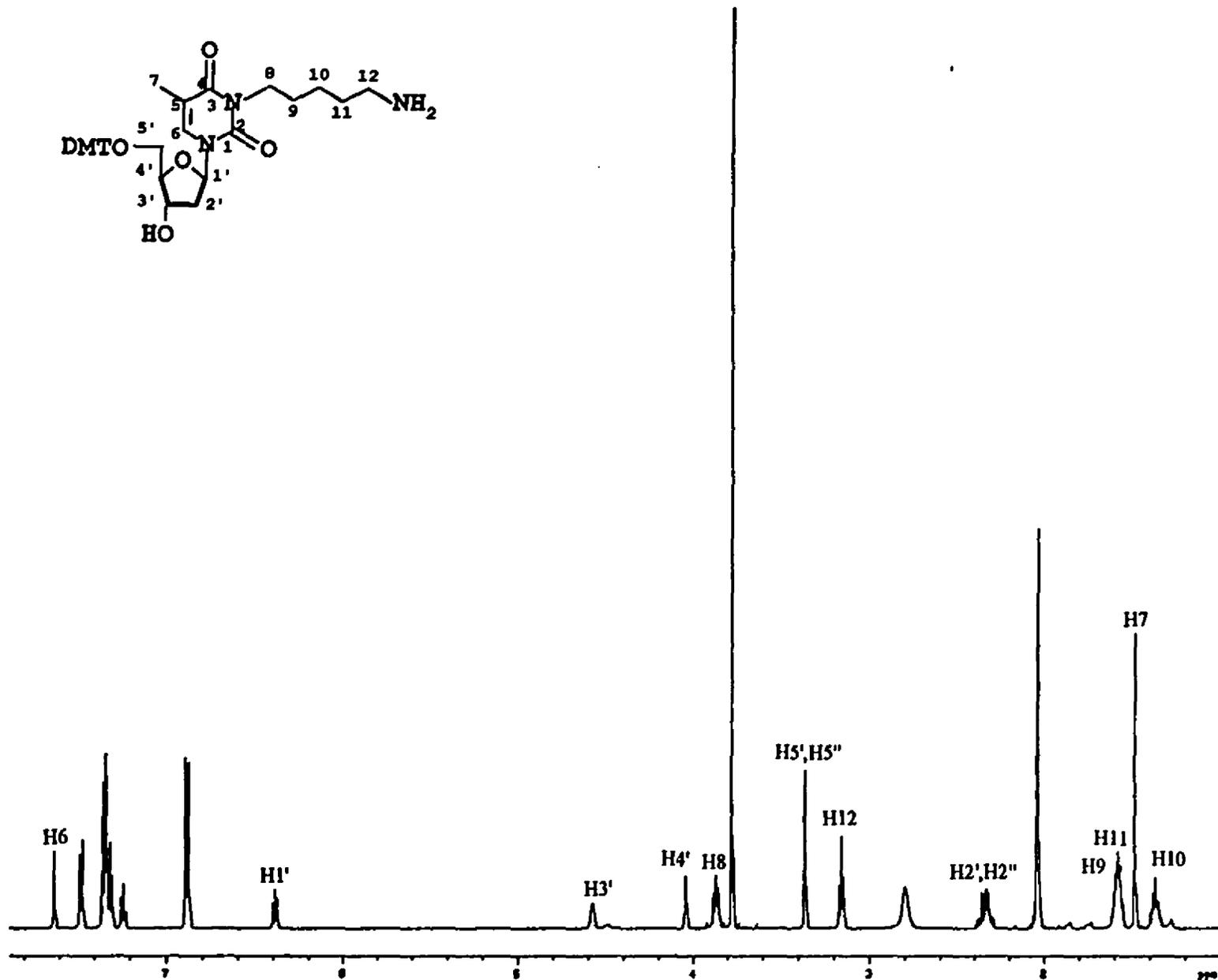
Figure 2.7 The 500 MHz <sup>1</sup>H-NMR spectrum of amino alcohol 12 in acetone-d<sub>6</sub>
