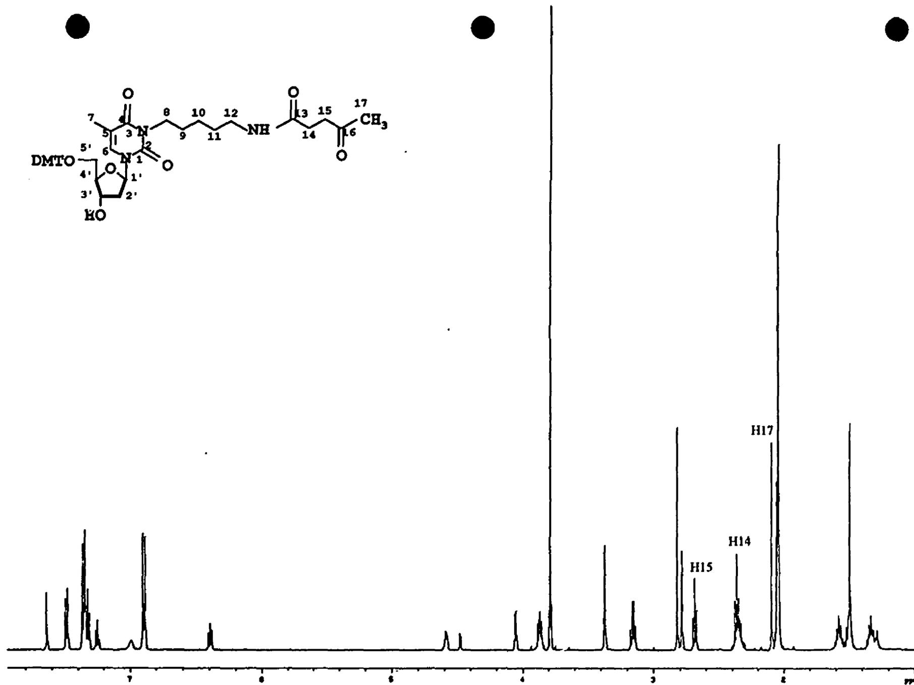
Figure 2.9 The 500 MHz <sup>1</sup>H-NMR spectrum of levulinic amide 16 in acetone-d<sub>6</sub>
