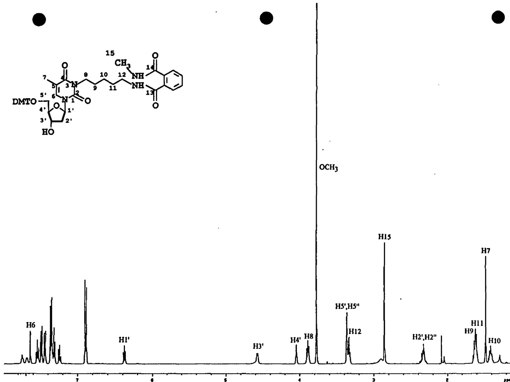
Figure 2.5 The 500 MHz  $^1\text{H}$ -NMR spectrum of phthalamide 11 in acetone- $d_6$
