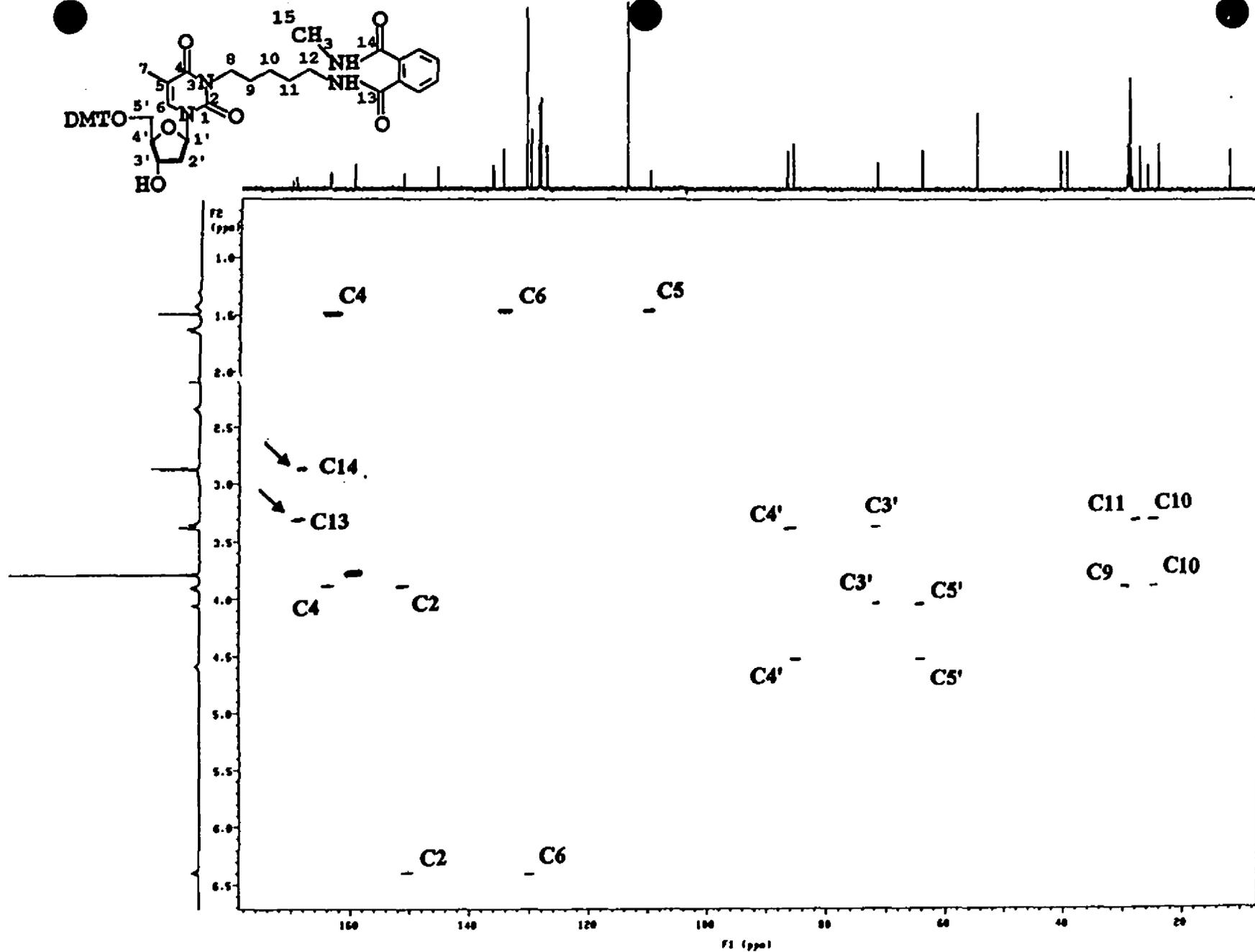
Figure 2.6 The 500 MHz HMBC spectrum of phthalamide 11 in acetone-d<sub>6</sub>
