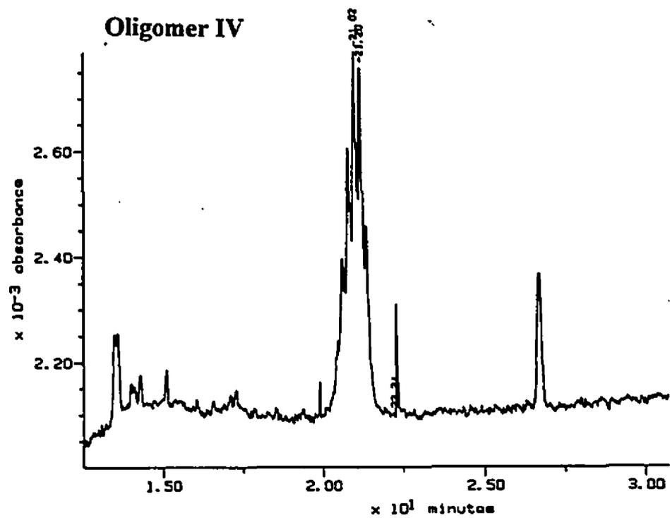
**Figure 4.2** Capillary Gel Electrophoresis Analysis of "Y"-shaped Oligomers III and IV after PAGE Purification
