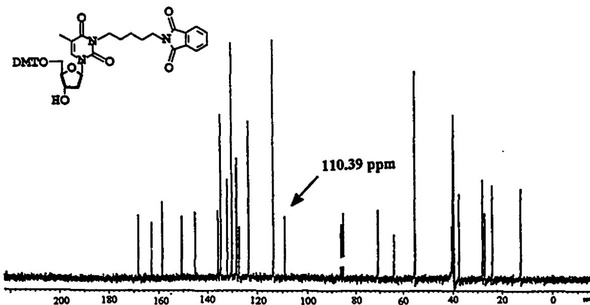
Figure 2.3 The 500 MHz  $^{13}\text{C}$ -NMR spectrum of 5 and 7. The C5 resonance signal is indicated. (for other assignments see table 2)
