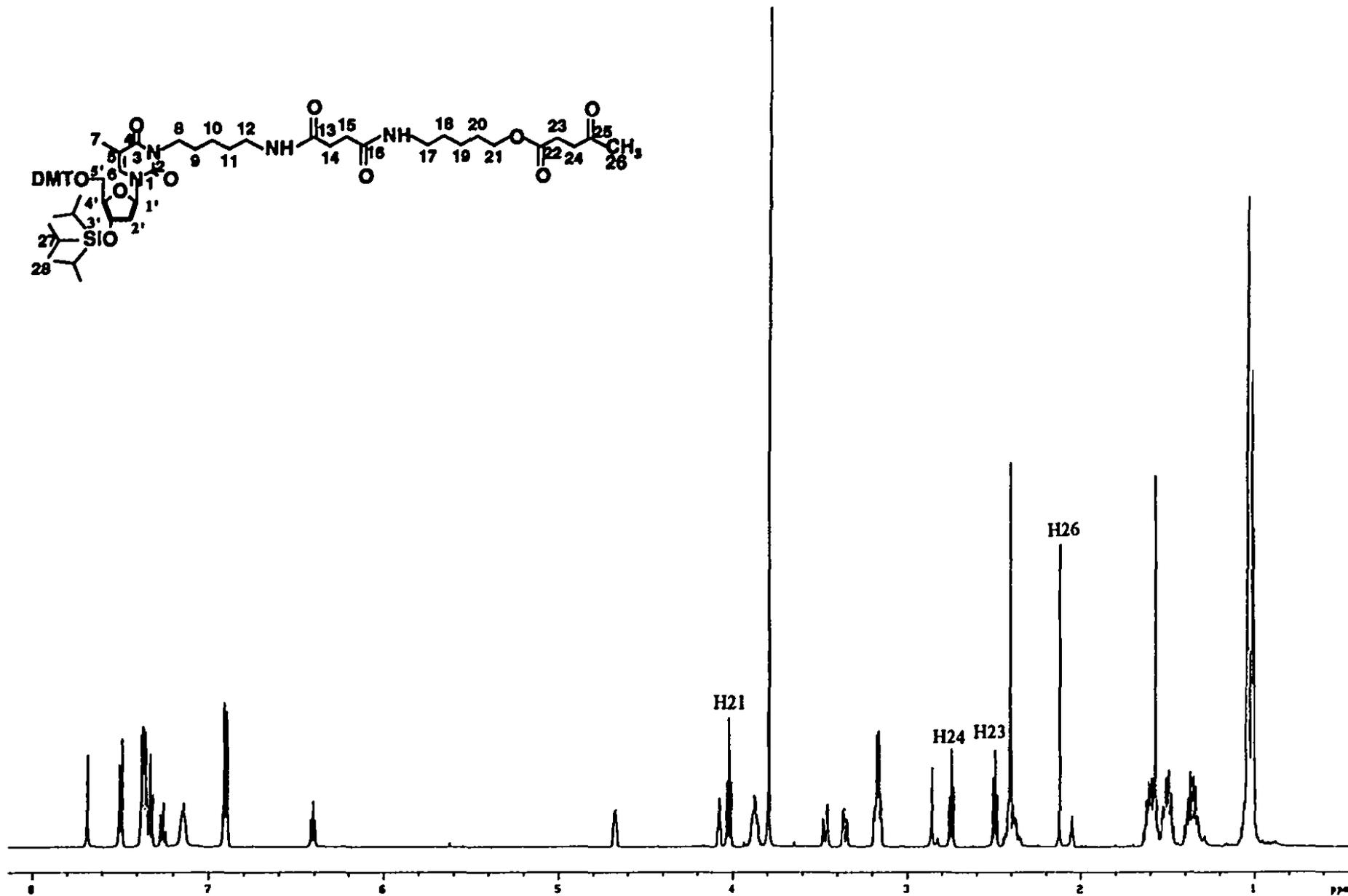
Figure 3.5 The 500 MHz <sup>1</sup>H-NMR spectrum of levulinic ester 34 in acetone-d<sub>6</sub>
