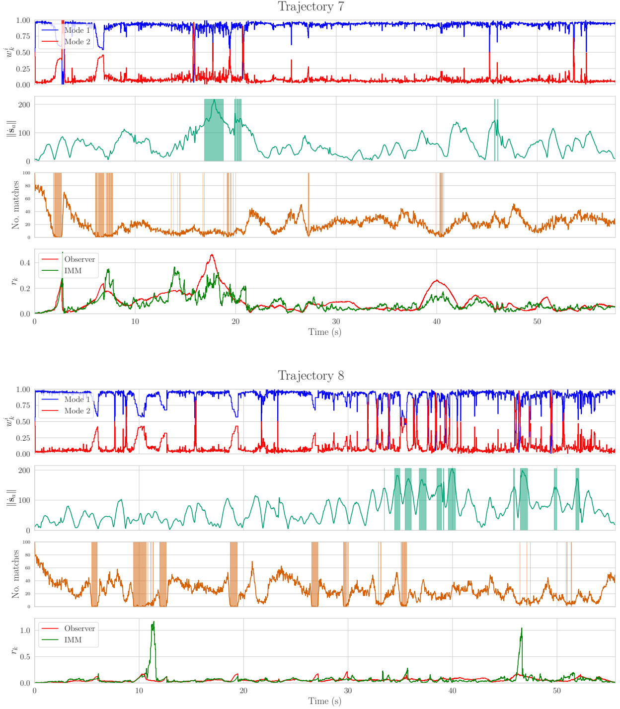
Figure 5.9: IMM model probabilities depending on how the \mathbf{s}_a is constant assumption is broken and number of matches in Trajectories 7 and 8. Mode 1 corresponds to \sigma_m^2 = 10^{-6} and mode 2 corresponds to \sigma_m^2 = 1 . Evolution of IMM and observer's error r_k is shown in bottom plots. Green shaded regions represent time frames where \|\dot{\mathbf{s}}_a\| > \alpha = 155 . Orange shaded regions represent time frames where number of tracked features goes below 4. When \|\dot{\mathbf{s}}_a\| > \alpha , the observer performance suffers. When insufficient features are tracked, the IMM performance suffers.
