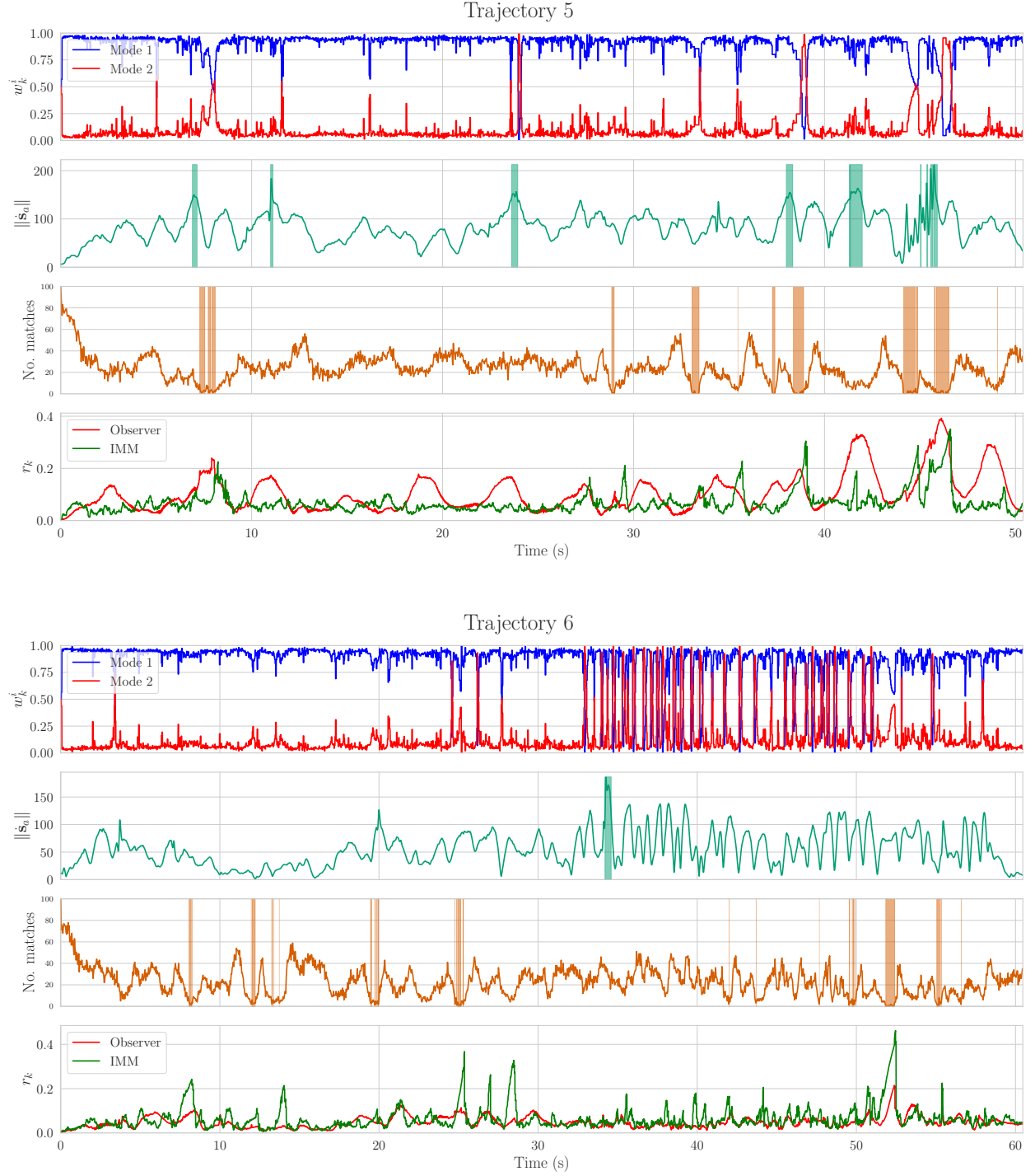
Figure 5.8: IMM model probabilities depending on how the \mathbf{s}_a is constant assumption is broken and number of matches in Trajectories 5 and 6. Mode 1 corresponds to \sigma_m^2 = 10^{-6} and mode 2 corresponds to \sigma_m^2 = 1 . Evolution of IMM and observer's error r_k is shown in bottom plots. Green shaded regions represent time frames where \|\dot{\mathbf{s}}_a\| > \alpha = 155 . Orange shaded regions represent time frames where number of tracked features goes below 4. When \|\dot{\mathbf{s}}_a\| > \alpha , the observer performance suffers. When insufficient features are tracked, the IMM performance suffers.
