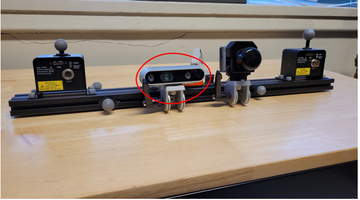
Figure 4.1: Front view of an Intel Realsense D453i, shown by the red circle, used to obtain both camera and angular velocity measurements. It is mounted on an T-slot aluminum profile. The numerous small gray spheres are the markers that the OptiTrack system uses to track the sensor head and generate ground truth data.
