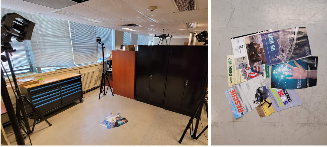
Figure 4.2: The experimental setup. The Intel Realsense D435i is moved in this space, observing the pages spread in the floor, employed to generate distinctive features on a plane. The OptiTrack system tracks the sensor head maneuvering in this space. A close-up of the tracked plane is shown in the right image.
