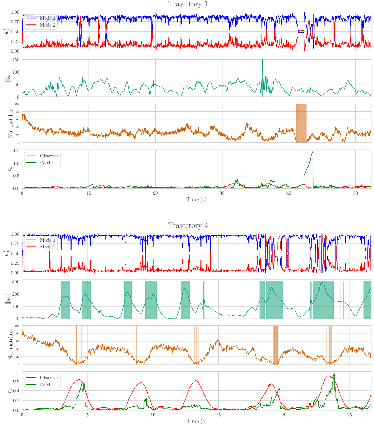
Figure 5.7: IMM model probabilities depending on how the \mathbf{s}_a is constant assumption is broken and number of matches in Trajectories 1 and 4. Mode 1 corresponds to \sigma_m^2 = 10^{-6} and mode 2 corresponds to \sigma_m^2 = 1 . Evolution of IMM and observer's error r_k is shown in bottom plots. Green shaded regions represent time frames where \|\dot{\mathbf{s}}_a\| > \alpha = 155 . Orange shaded regions represent time frames where number of tracked features goes below 4. When \|\dot{\mathbf{s}}_a\| > \alpha , the observer performance suffers. When insufficient features are tracked, the IMM performance suffers.
