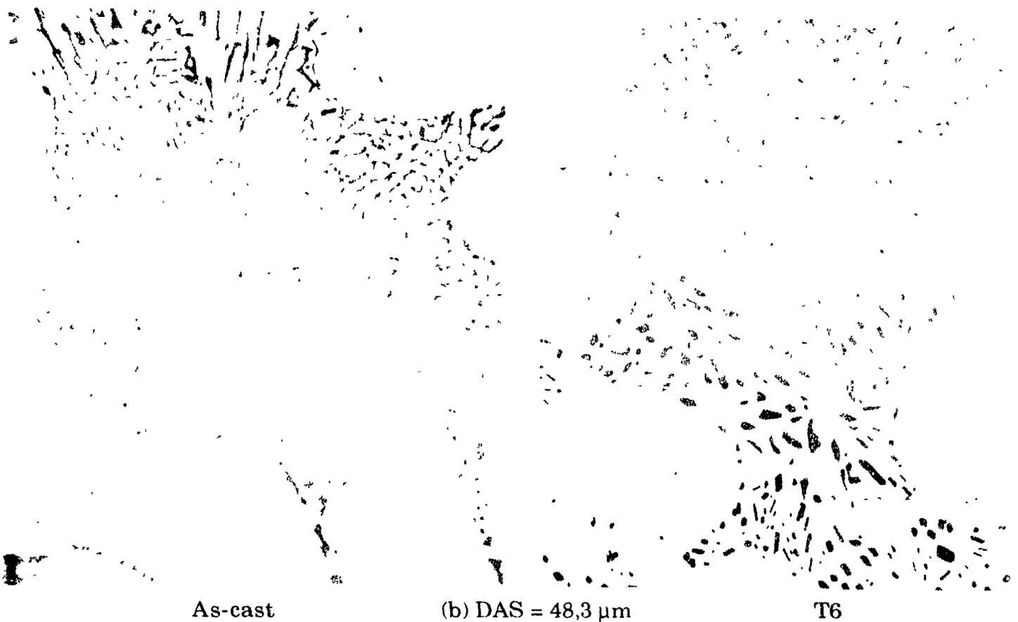
***Figure 4.13 : Micrographs of as cast and T6 unmodified Al-Si alloy
