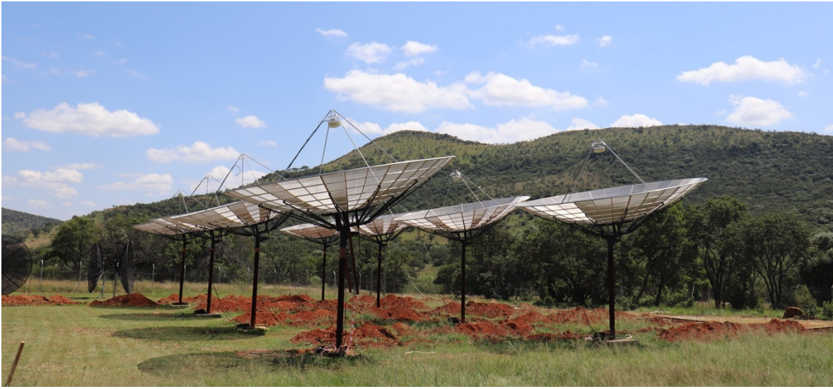
Figure 2.3: 8-dish prototype set up at HartRAO site. Dishes displayed are one of the prototypes which are being tested, other dish prototypes also exist but are not included in this photograph. Photo credit HIRAX Facebook page [21]
