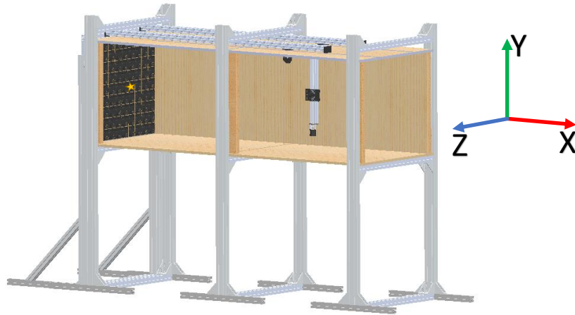
Figure 3.2: CAD of wind tunnel with traversing mechanism, side wall removed. Figure also shows coordinate system used. The origin (0,0,0) is located at the center of the face of the center fan, the yellow star in the figure
