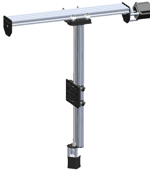
Figure 3.3: Planar traversing Mechanism for the wind tunnel.
