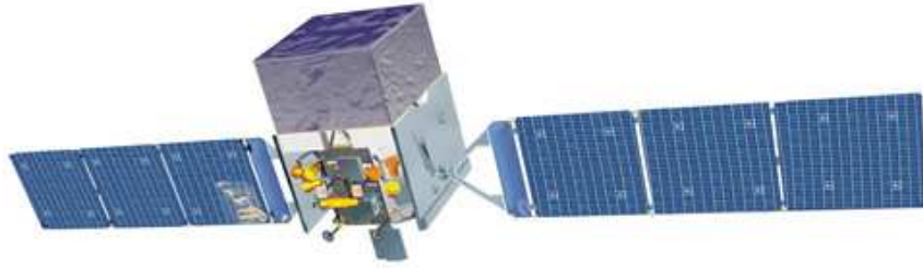
Figure 3.4 An artist's impression of Fermi . The large silver rectangular prism on the top is the LAT, and the yellow cylinders in the bottom are the GBM. Image from heasarc.gsfc.nasa.gov/mission_pages/GLAST/multimedia/ .
