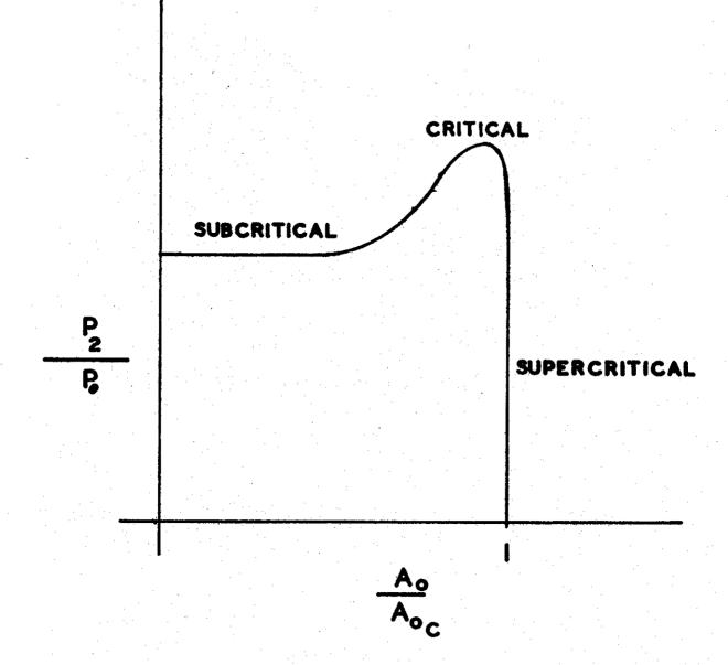
FIG.3 TYPICAL DIFFUSER PERFORMANCE CURVE
