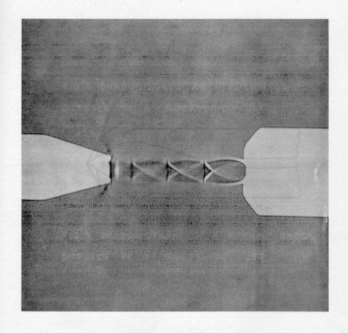
FIG. 5 SHADOWGRAPH OF A NORMAL SHOCK DIFFUSER IN A SUPERSONIC JET.
