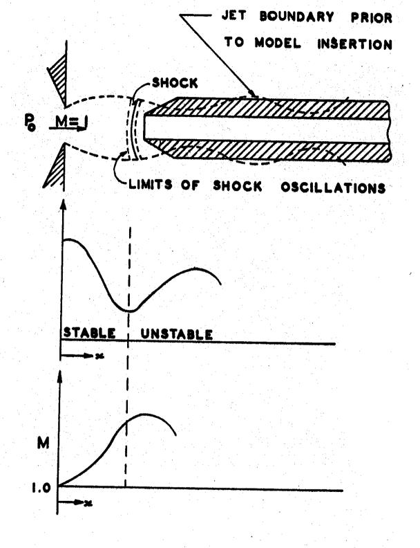
FIG. 4 CHARACTERISTICS OF THE HARTMANN SOUND GENERATOR
