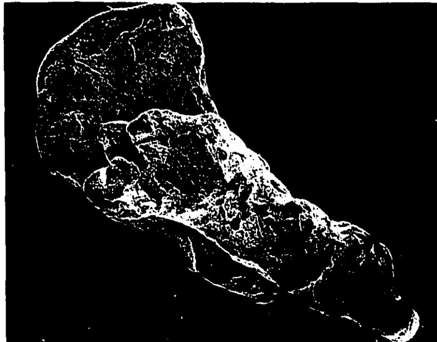
**Figure 5.22:** A folded and flattened lead fragment recovered from the Bond rod mill (feed size: 0.850-1.000 mm).
