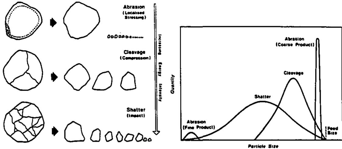
**Figure 2.1:** Representation of the mechanisms of particle fraction and the resulting product size distributions (reprinted with permission from Kelly and Spottiswood<sup>(39)</sup>).
