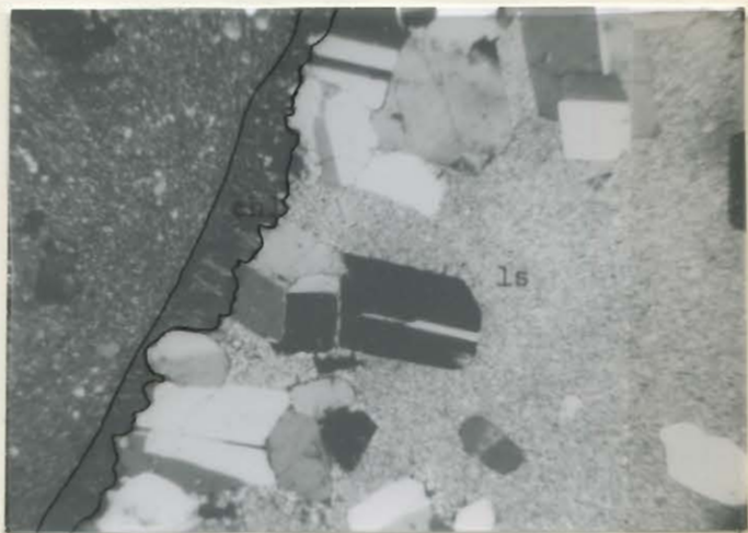
Fig. 2 Authigenic, euhedral albite crystals growing into a limestone(ls) clast. Outer rim is chlorite(chl). X 20 Low. Rapitan, Section UB 3, 126 feet above base of section.
