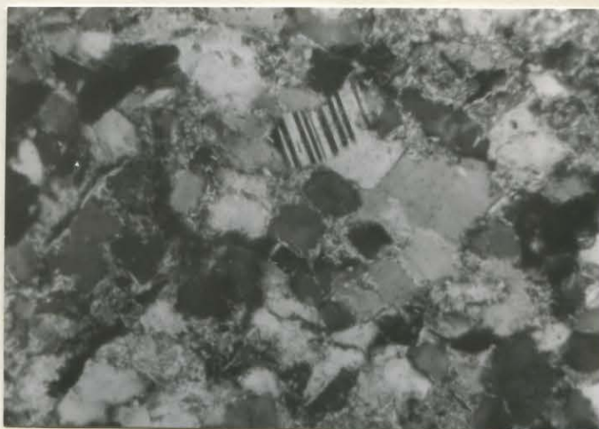
Fig. 2 Poorly sorted arkose. Quartz, orthoclase and minor plagioclase grains in sericitized clay matrix. X 20 Upper Rapitan, Section UB 3, 5,617 feet above base of section.
