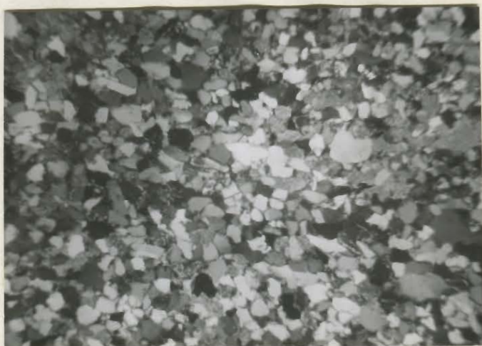
Fig. 3 Upper Rapitan arkoses. Note subangular to subrounded poorly sorted grains. Matrix is subordinate.
