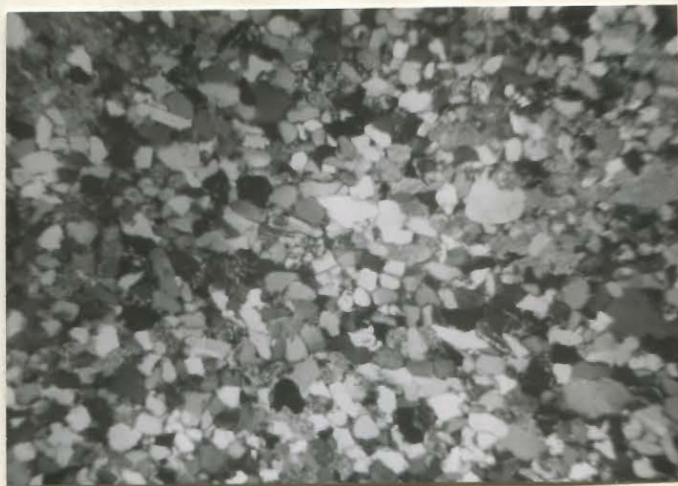
Fig. 3 Upper Rapitan arkoses. Note subangular to subrounded poorly sorted grains. Matrix is subordinate. X 20 Upper Rapitan, Section UB 1, 5,945 feet above base of section.
