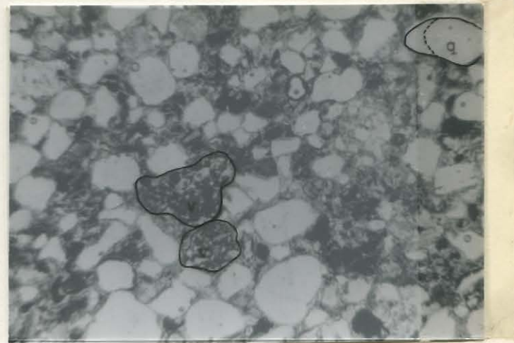
Fig.3 Lithic sandstone. Poorly sorted subangular to rounded quartz and feldspar grains, minor shale or mudstone clasts, two volcanic(v) fragments. Quartz overgrowth upper right(q). X 20 Low. Rapitan, Section UB 3, 300 feet above base of section.
