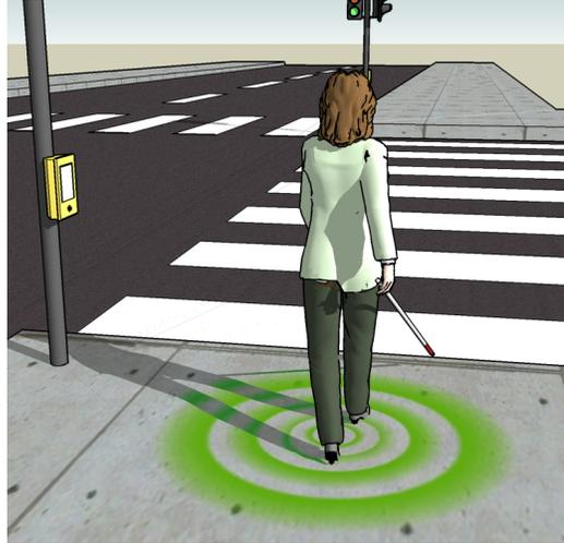
**Fig. 3.1** A possible end-user scenario: Pedestrians receive vibrotactile cues via the ground surface, indicating the location of the crossing and state of its signal.
