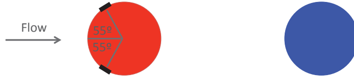
Figure 3–4: Schematic showing the location of the boundary layer trips in the tandem cylinder wind tunnel experiment.
