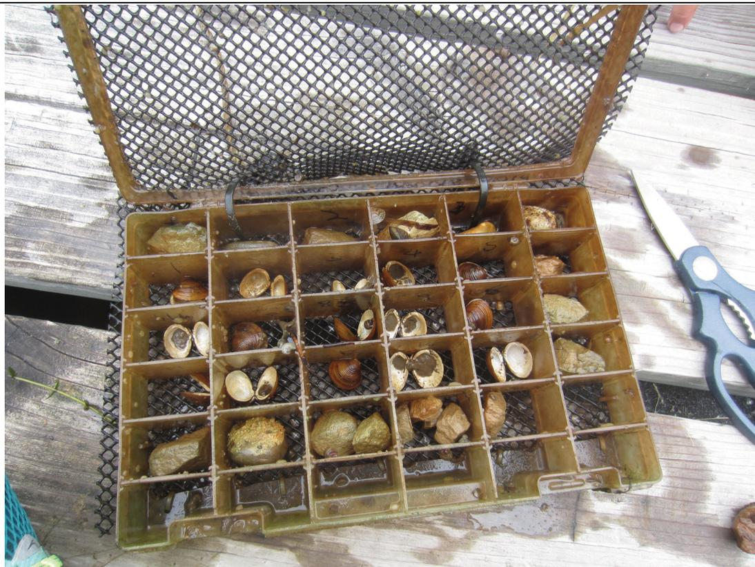
Figure 3.3: Experimental units within which shells were stored during deployment periods. Pictured here is a unit containing Upper Clinch River clam shells deployed at Site Y in Test 2, after collection in August 2015.
