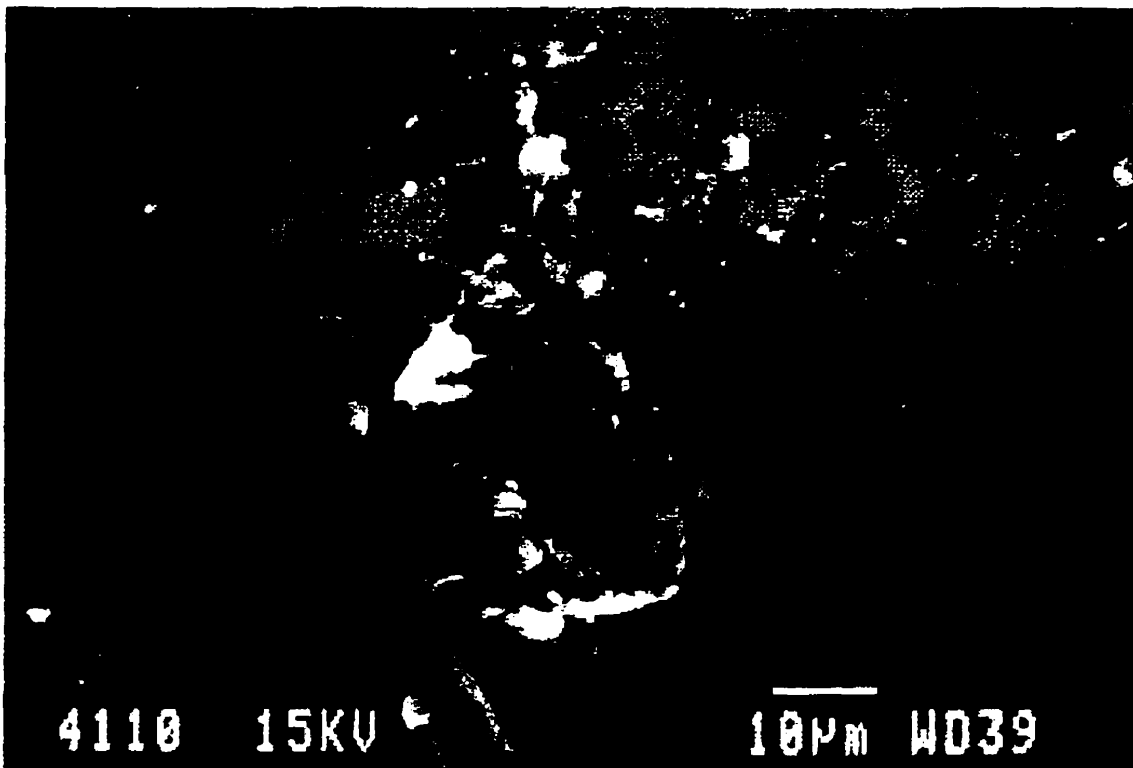
Figure 5.49 - Salt deposit on a Photoresist Surface
