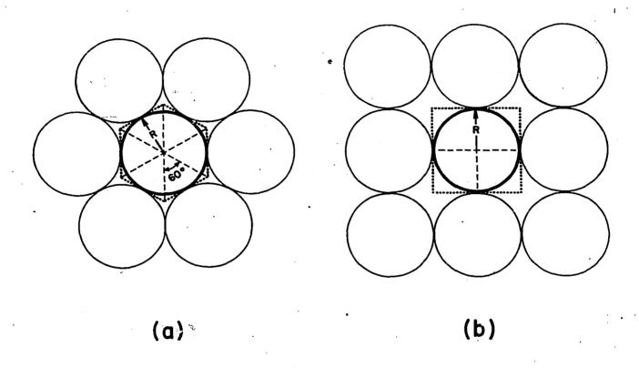
Figure III. Hexagonal (a) and cubic (b) close packing of spheres. It is evident from mere inspection that the packing in the former is more efficient than in the latter. To calculate the fraction of the total area occupied by spheres resting on a horizontal surface it is necessary to find the areas of the respective circumscribed hexagon and square shown in the figure.
