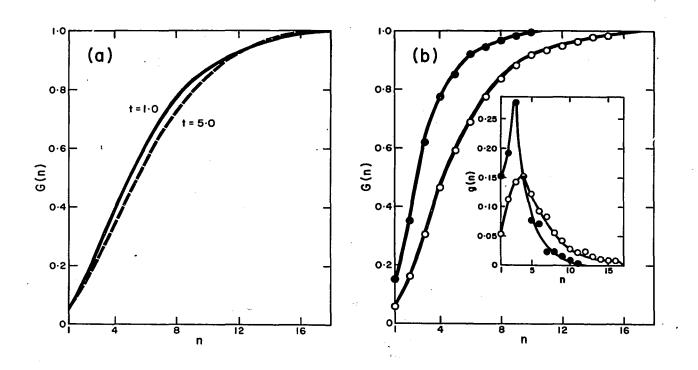
Figure 6. (a) Change in particle number distribution with time (minutes) for steel rods  $r_p = 5.97$ , c = 0.82 on a solid surface at 10 vibrations/second.
