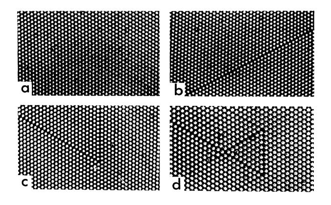
Figure 11. Linear dislocations arising from the vibration of a hexagonally close-packed monolayer of spheres. (a) Close-packed layer, c.f. Figure 1b. (b) Dislocations in adjacent rows. (c) Dislocations meeting at 600 to produce V-structure. (d) Formation of  $\Delta$ -structure through meeting of 3 dislocations at 600.
