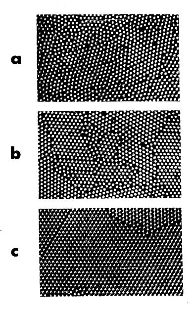
Figure 10. The effect of vibrations on the size of crystallites of hexagonally close-packed spheres (ball bearings 0.48 cm. diameter) resting on a solid surface. The photographs show a central domain of the plate. (a) t = 0; small crystallites separated by grain boundaries can be seen. (b) t = 1 min. (c) t = 2 min. after vibration started: the crystallites increase in size at the expense of the grain boundaries and the surface concentration has grown from 0.41 in (a) to 0.81 in (c).
