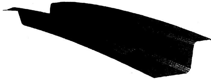
Figure.7.1: Deformed reverse position panel at 24kPa.
