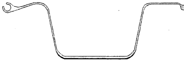
Profile E: Reverse design with increased compressive plate thickness
