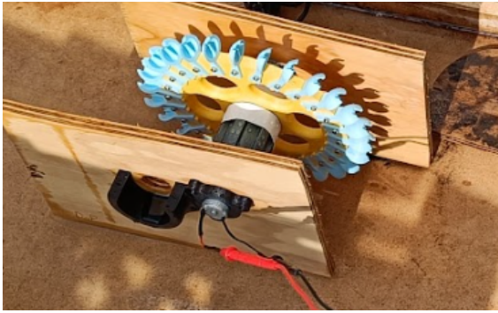
Figure 32. Mounting of the turbine
