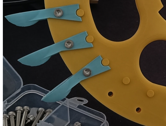
Figure 18. Buckets mounted on the big turbine.
