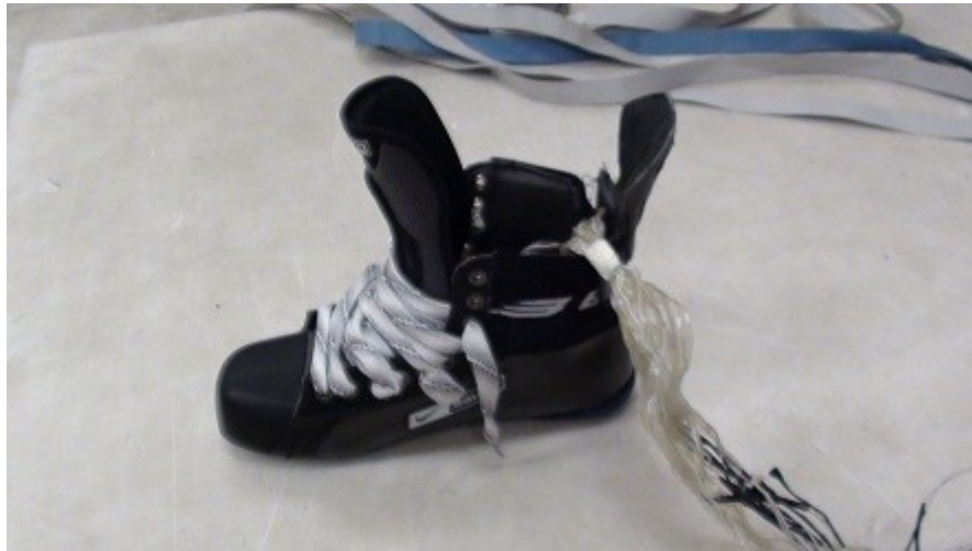
Figure 3.8: COP measurement system inside the boot
