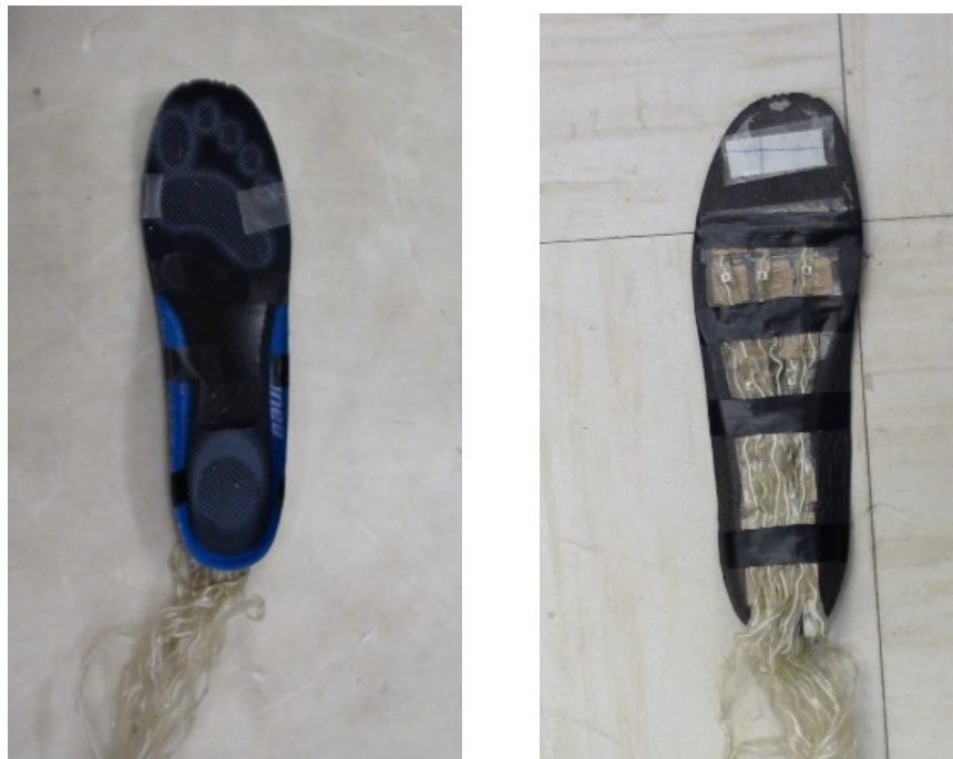
Figure 5: FSA sensors fitted under the insole
