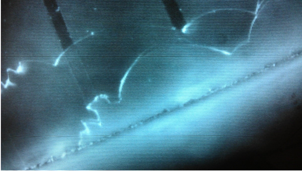
Figure 20: The dicing was moved closer to the waveguides and the results were much worse. The two layers of Chalcogenide glass can be seen chipped away at different positions. The gold layers are stripped much farther back from the edge.
