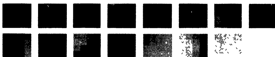
Figure 4.10: Codebook of a memoryless VQ using 16 codevectors and the edge weighted distortion measure, optimized on the image of Lenna.
