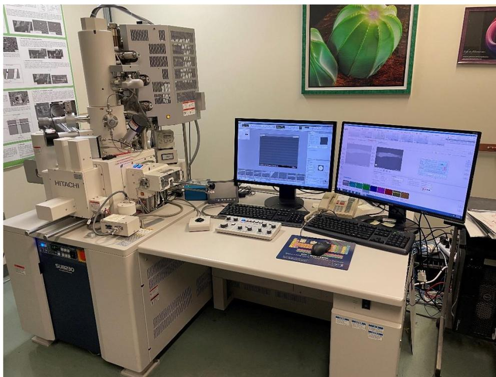
**Figure 3.7:** The SU8230 microscope utilized for obtaining SEM and EDX images.
