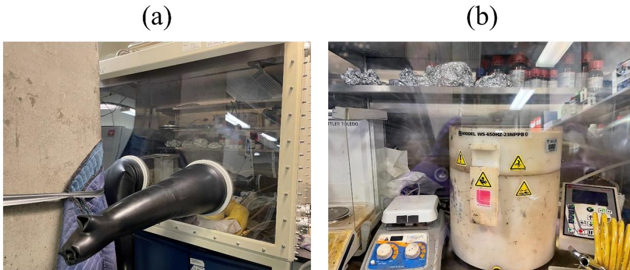
**Figure 3.4:** (a) The nitrogen-filled glovebox utilized for making the precursor and synthesizing perovskite layer as well as HTL. (b) the spin coater and hot plate/stirrer inside the glovebox.
