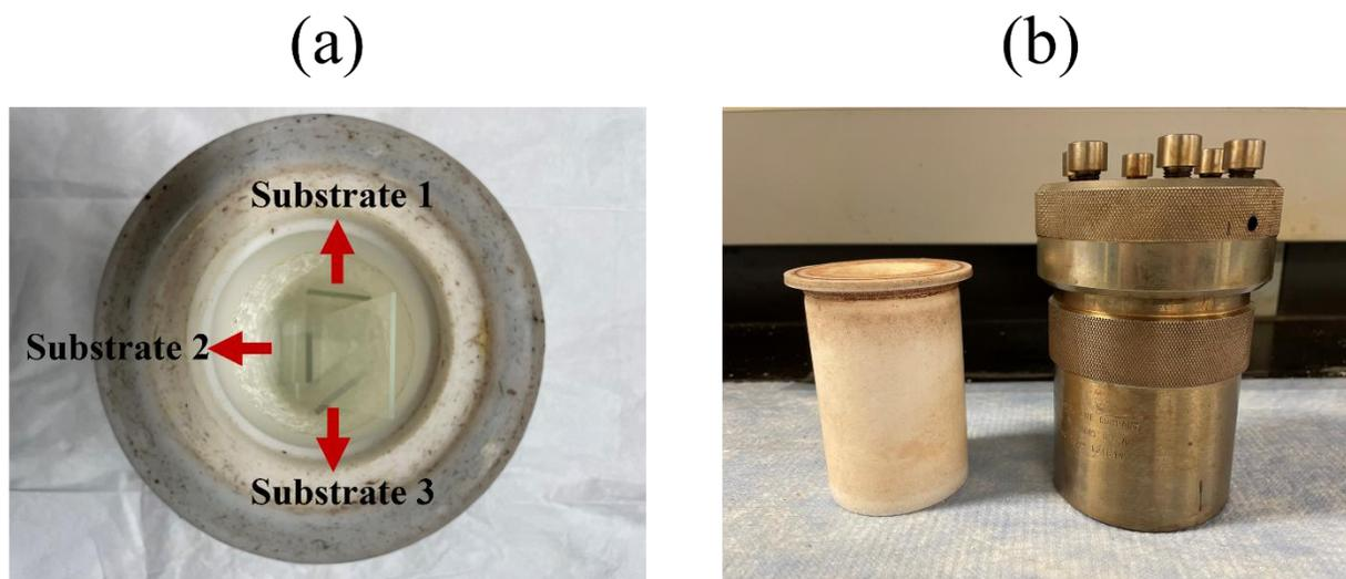
**Figure 3.2:** (a) Arrangement of the substrates inside the Teflon lining, (b) the Teflon lining (left) is then sealed inside the metal encasing (right) and placed inside the oven for hydrothermal synthesis.
