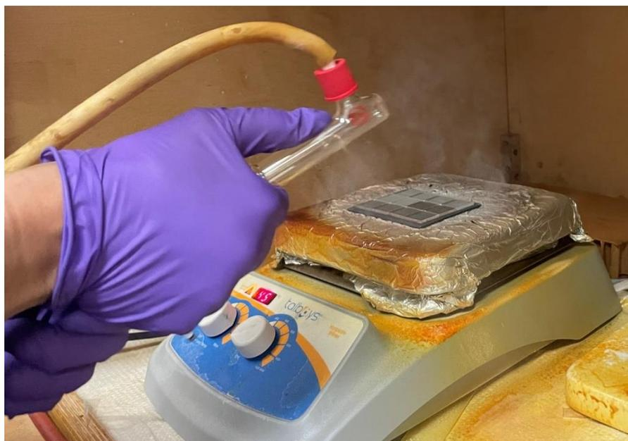
**Figure 3.3-** The spray pyrolysis setup.
