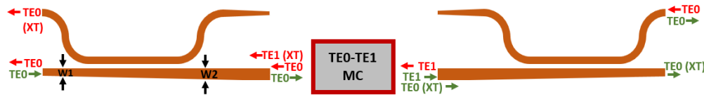
Fig. 3.2 Schematic of the circuit block for device characterization, showing the forward (in green) and reverse (in red) propagation through the TE0-TE1 mode converter.
