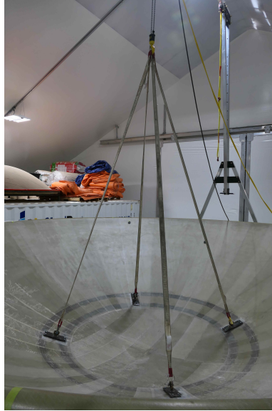
Figure 3.26: First D3A six meter dish partially supported by a crane attaching to the future feet locations of the feed legs.
