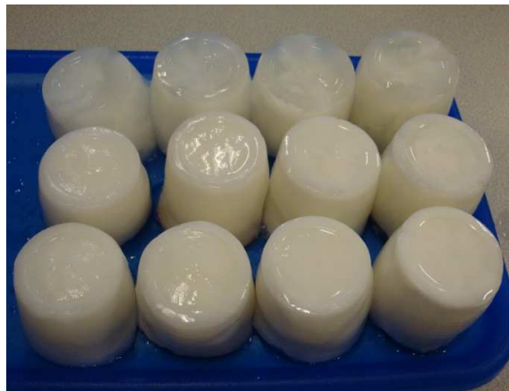
Figure 4-1: Samples of PVA-C from 4-8% (left to right) and 1-3 freeze-thaw-cycles (top to bottom). Note that the samples that have undergone 1 freeze-thaw-cycle (FTC) samples are more translucent than higher FTC samples. Note that the 4% 1 FTC sample is deforms significantly under its own weight.
