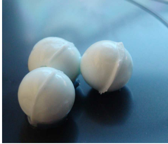
Figure 4-4: The 11–12 mm diameter multimodal spherical markers implanted into our phantom
