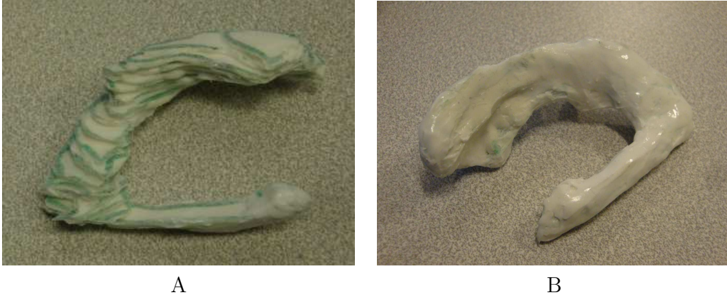
Figure 4-3: The silicone rubber and cellulose composite mold component used to cast the fluid filled left ventricle in our phantom (A) before and (B) after being covered with additional silicone caulking to smooth the surface.
