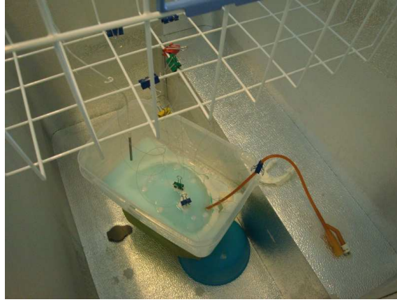
Figure 4-5: The setup for casting the hemispheric portion of the phantom. After the hemispheric part is well frozen, the clamps are removed and PVA solution for casting the base is poured into the mold.
