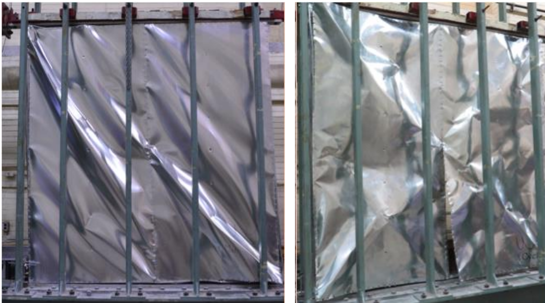
Figure 2.19 Shear Buckling and Tension Field of Sheathing ; a) Monotonic Test (1830 × 2440 mm (6' × 8')), b) Reversed Cyclic test (1830 × 2440 mm (6' × 8'))
