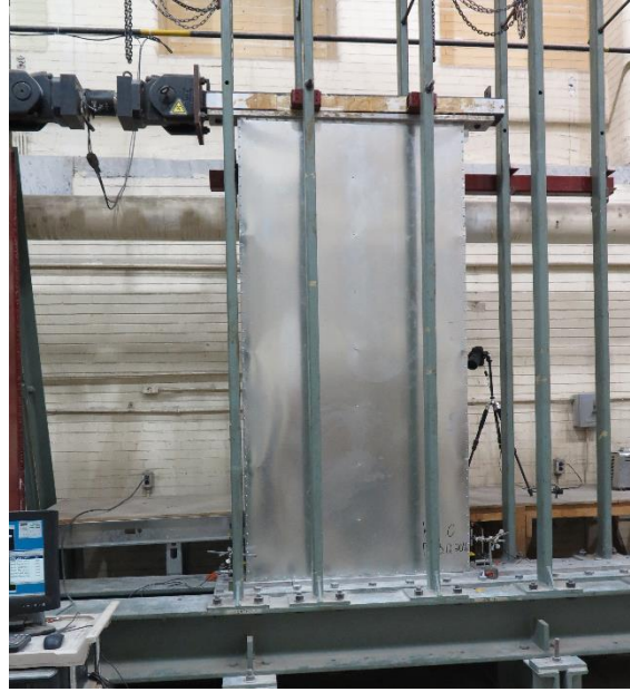
Figure 2.2 Typical wall installation in test frame
