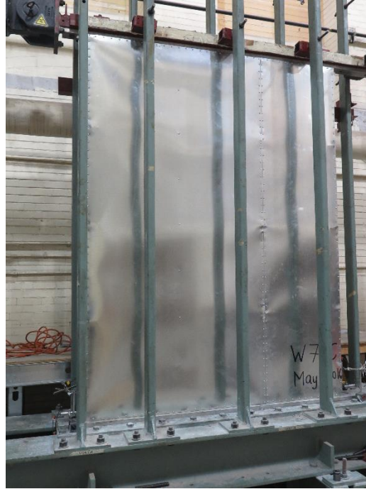
Figure 2.7 Sheathing combination for 1830×2440 mm (6'×8') shear walls
