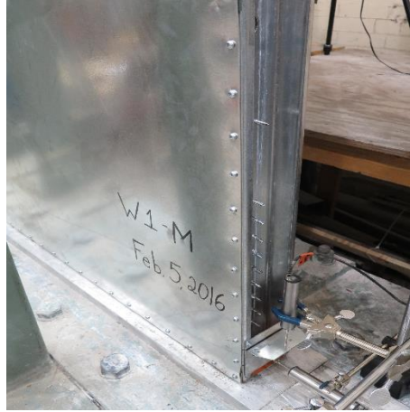
Figure 2.9 LVDT placement on non-structural steel plate
