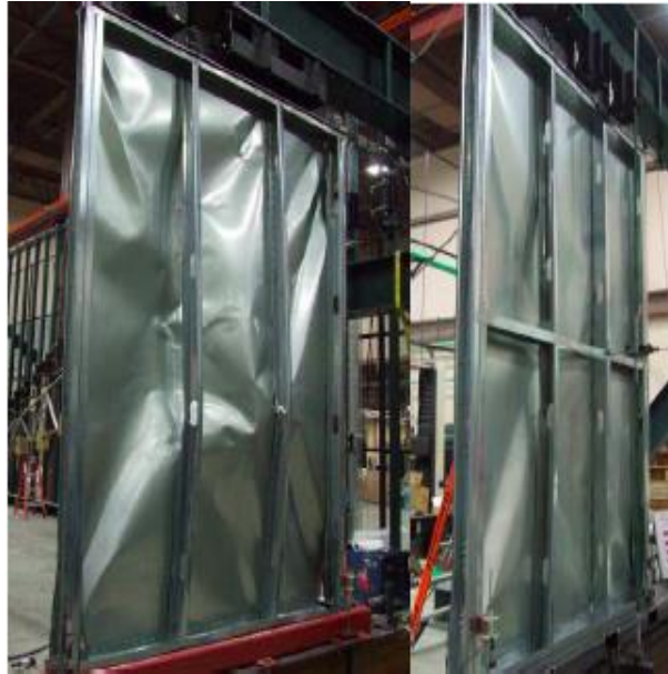
Figure 1.2 Failure mode of 6'x8' wall with (right) and without (left) special detailing (Yu et al., 2009)
