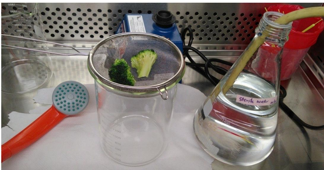
**Figure 17:** The spraying unit/shower head at left corner (orange in colour) was used for the spraying of CPC solutions onto food samples
