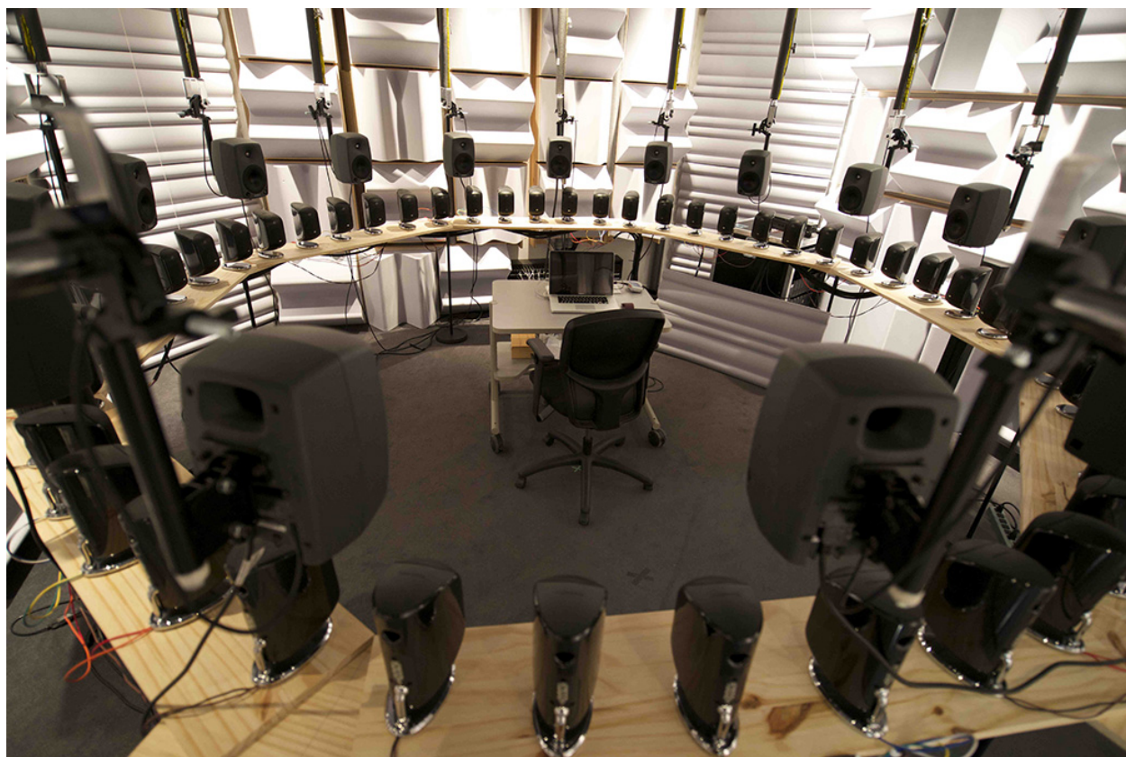
Figure 5.1: Loudspeaker array and listener position in the first experiment. Only the larger loudspeakers in the upper circle (Genelec 8030) were used, the smaller loudspeakers are part of another experiment. In addition, four height channels were used, which are not shown in this photograph.
