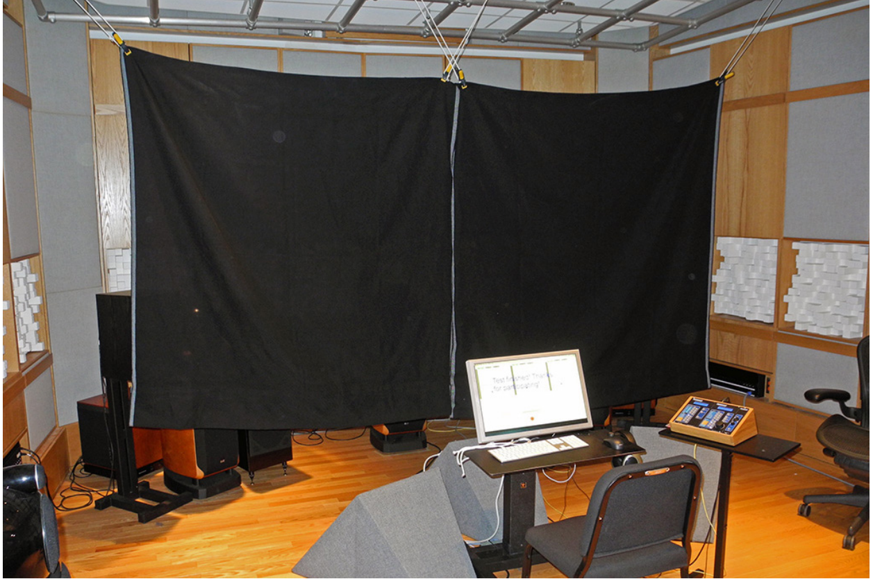
Figure 5.5: Test setup in the second experiment. The frontal loudspeakers were hidden by the acoustically transparent curtain. The lights in the room were dimmed so that the walls and ceiling behind the curtain were not visible from the observation position.
