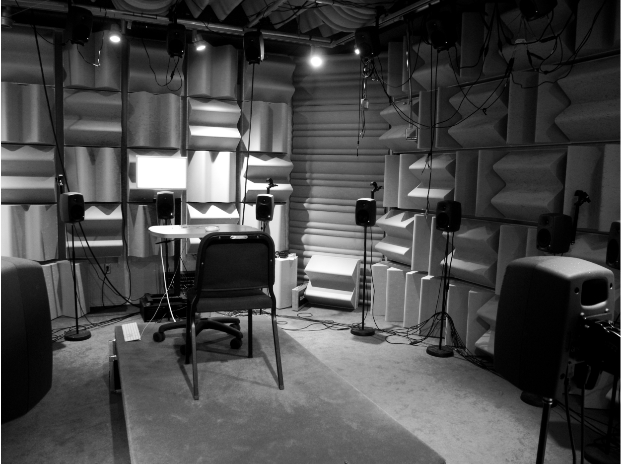
Figure 3.1: Experimental apparatus used for the listening test consisting of two rings of Genelec 8020A loudspeakers. The participants sat on a riser platform in the middle of the setup to be aligned with the high-frequency drivers of all loudspeakers. Subsequent signal measurement using a dummy head as well as a B-Format microphone were done in approximate position of the participant’s head.
