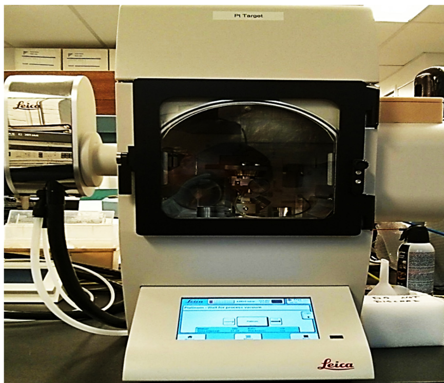
Figure 5-9-Sample preparation for the scanning electron microscopy. The chitosan fiber is not an electrical conductor and required a platinum coating.
