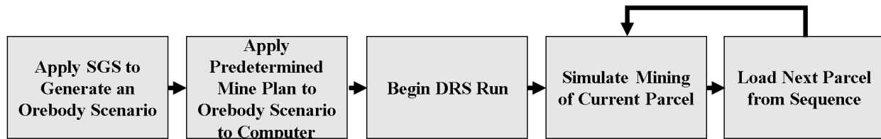
Figure 3.3.2: Geostatistical approach, in which geological data is generated prior to the execution of the DRS, through Sequential Gaussian Simulation.
