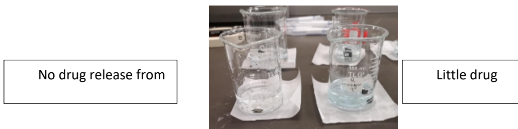
Figure 3-29: Comparison between Fe-SS with CNTs and without CNTs, we see on the right little drug release while on the left image there is no drug release.
