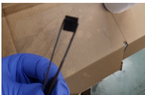
Figure 3-12: Image of Fe-SS sample after the growth of CNTs, with etching for 15 minutes and 10 minutes of acetylene injection
