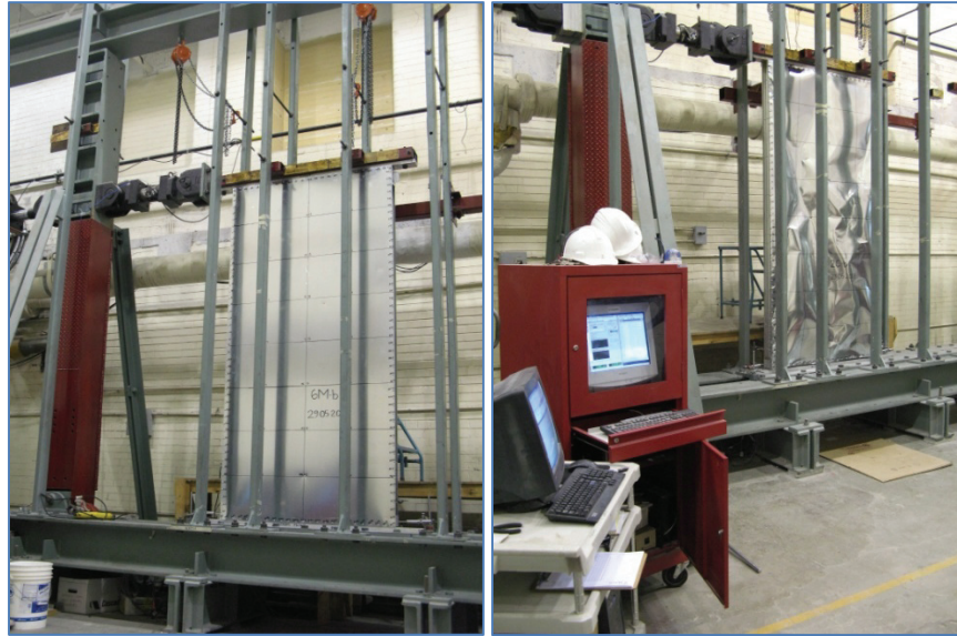
Figure 2.2 Wall Installation in Test Frame
