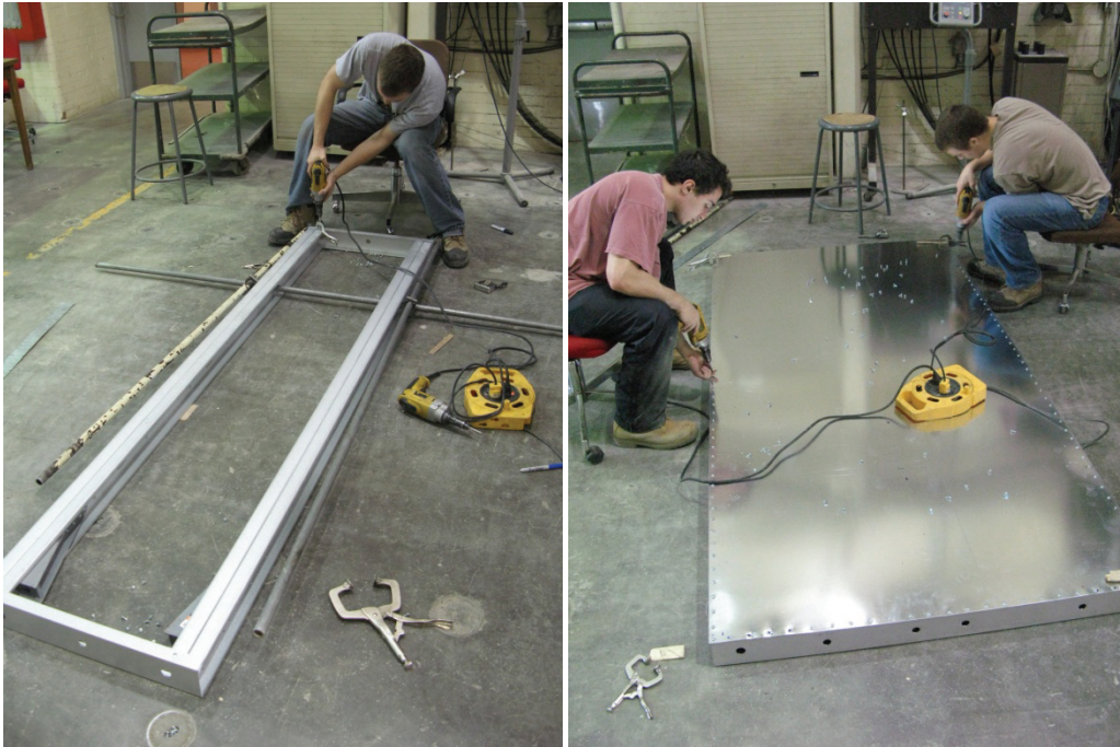
Figure 2.4 Frame and Sheathing Assembly
