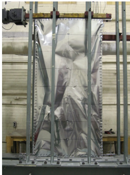
Figure 2.19 Shear Buckling and Tension Field of Sheathing in a Reversed Cyclic Test
