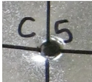
Figure 2.13 Screw Pull-Through Sheathing Failure
