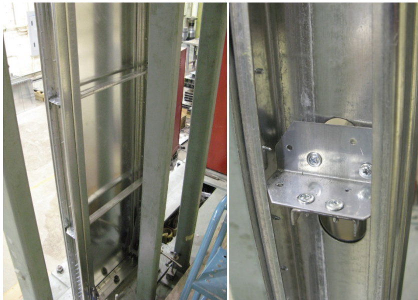
Figure 2.5 Bridging and Bridge Clip in Test 9M-c
