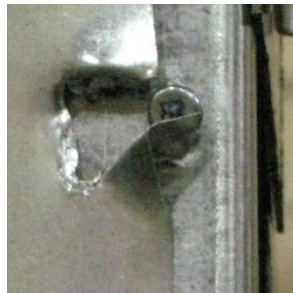
Figure 2.15 Screw Tear-out Failure
