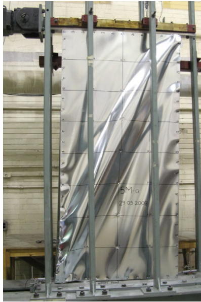
Figure 2.18 Shear Buckling and Tension Field of Sheathing in a Monotonic Test
