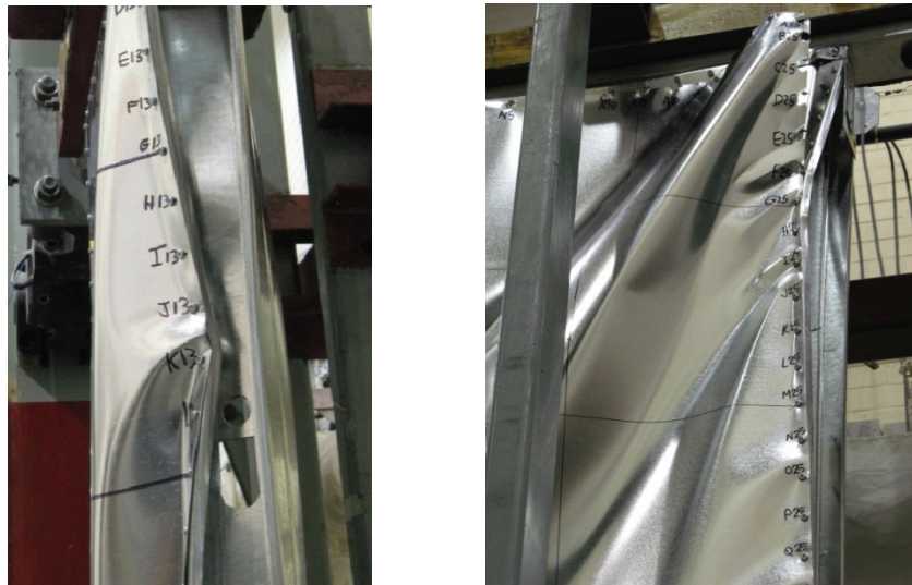
Figure 2.20 Twisting and Local Buckling of Chord Stud
