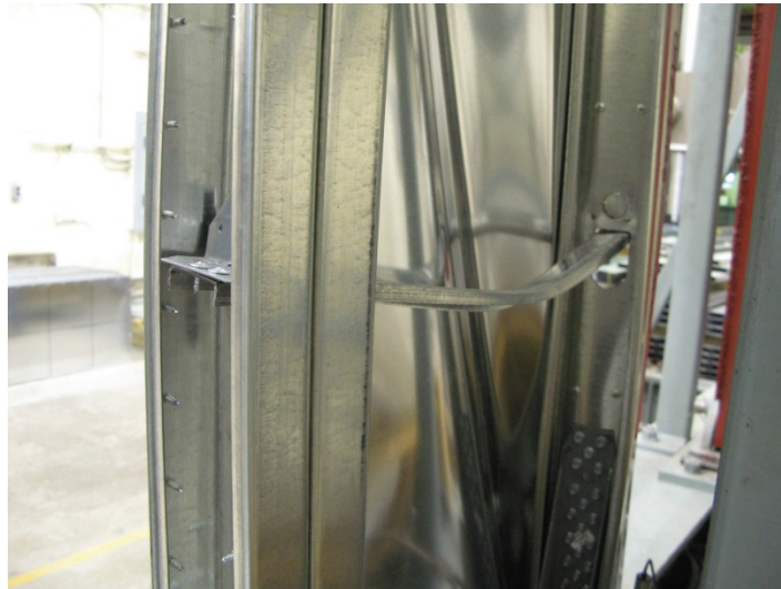
Figure 2.21 Flexural Buckling of Bridging in Test 9M-c
