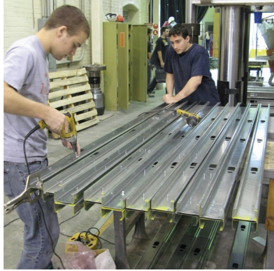
Figure 2.3 Chord Stud Assembly
