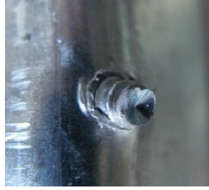
Figure 2.16 Screw Shear Fracture Failure
