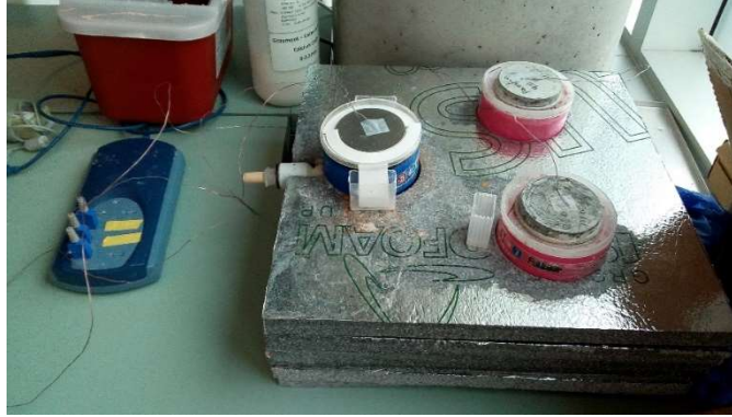
Figure 35: Thermocouples on the 3 heaters from the first prototype
