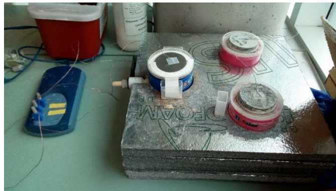
Figure 10: Three heaters for PCR reactions at different temperatures
