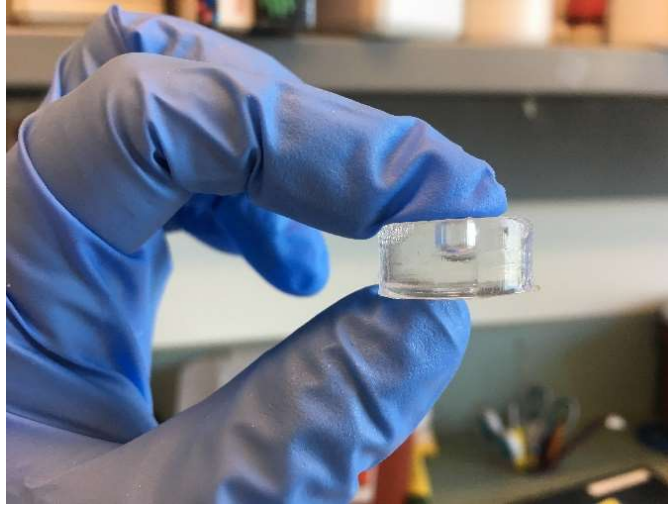
Figure 27: PCR Liquid inside PDMS
