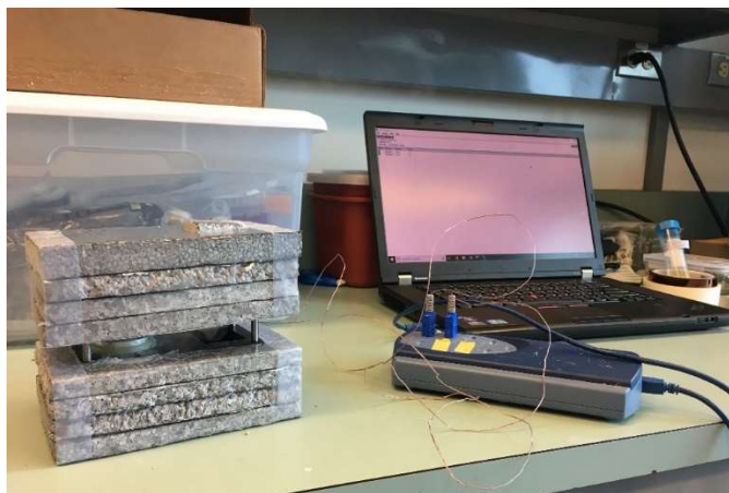
Figure 37: Setup with 2 thermocouples for data recording
