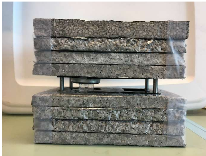
Figure 30: Gap in the middle layer
