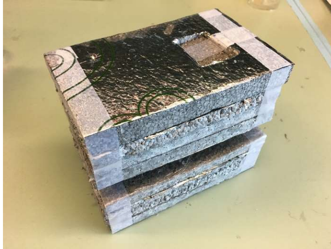
Figure 29: Insulation housing (1mm thick polystyrene panel)
