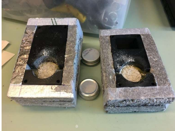
Figure 16: Magnesium-iron powder in a fuel holder
