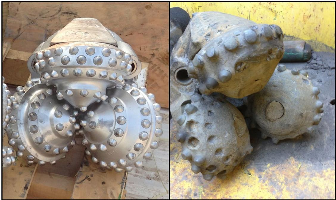
**Figure 4-42: Comparison of new and completely worn drill bit**
