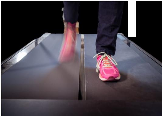
*Supplementary Figure 5.1: Split belt treadmill walking. Independently driven belts running at different speeds.*
