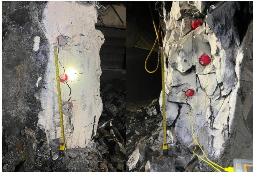
*Figure 7.18 Cracking Coalescing between SCDA holes of Slash #2*
