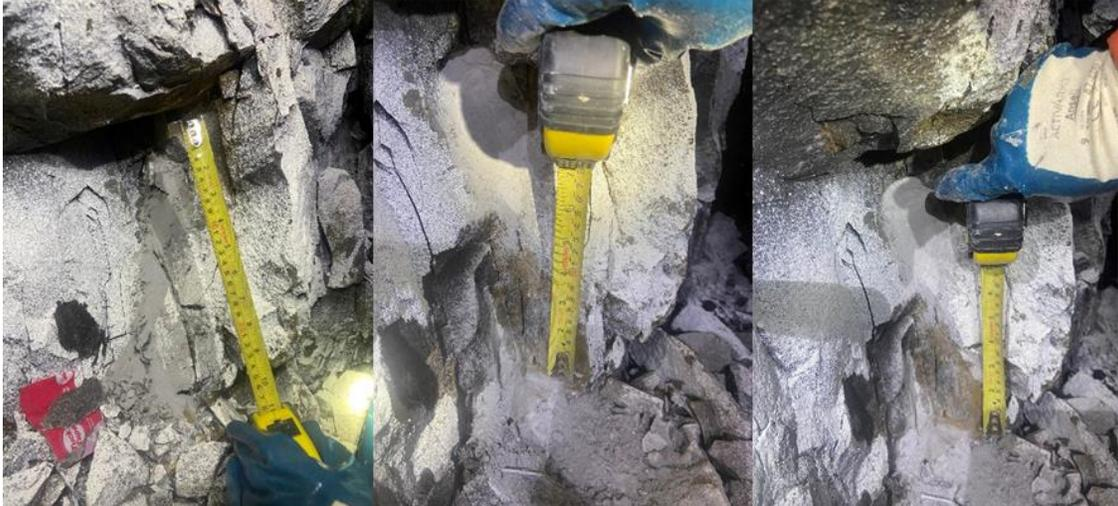
*Figure 7.16 Minimal cracking around bottom left hole of Slash #1*
