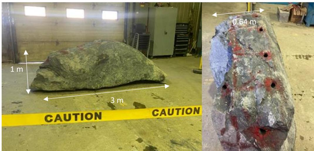
Figure 7.1 Greywacke boulder tested at Hoyle Pond mine site
