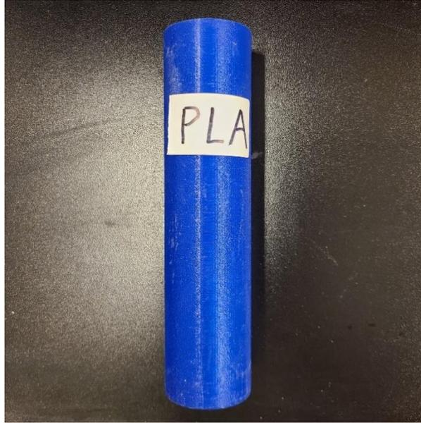
Figure 7.10 Plastic Cartridge used for horizontal loading of slash tests
