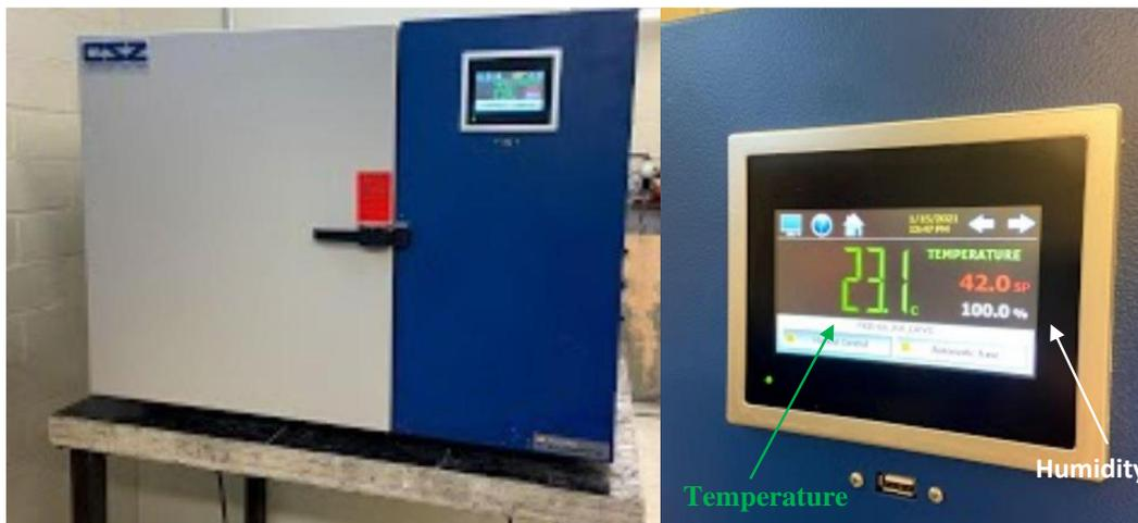
Figure 6.1 Microclimate benchtop chamber (Model #: MCB (H)-1.2).
