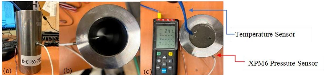
*Figure 3.6 Direct pressure measurement in specimen S-C-150-275-S with (a) Side view of XPM6-1KBG Miniature Pressure Sensor (b) Top view of XPM6-1KBG miniature pressure sensor threaded into wall cylinder (c) Expansive cement filled cylinder with embedded temperature sensor*
