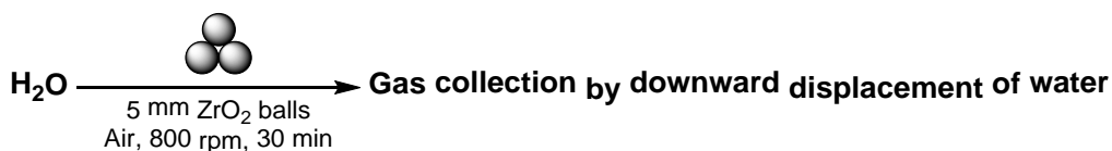
120 Table 1. Galvanic generation of H 2 gas by milling of water in a Ni- and Cr-containing stainless steel 121 assembly 55
