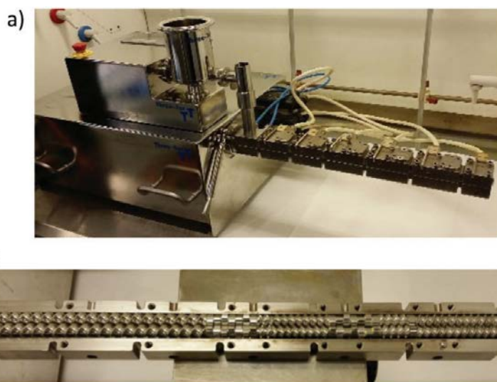
758 759 Fig 19. Twin screw extruder (TSE) apparatus employed for continuous, solid-state organic transformations 96
