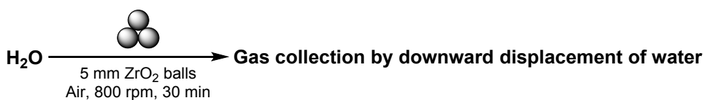
120 Table 1. Galvanic generation of H 2 gas by milling of water in a Ni- and Cr-containing stainless steel 121 assembly 55
