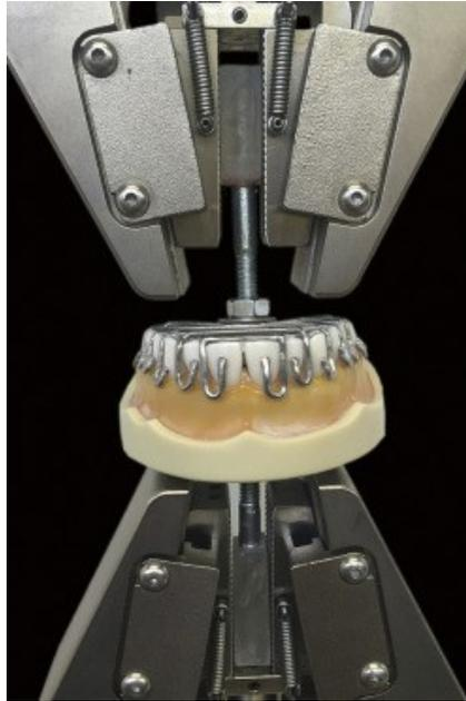
Figure 2-4: I-bar clasps engaging on teeth in a mechanical retention experiment [105].
