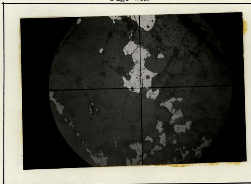
Pyrite along a quartz vein contact with ore "diorite" (reflected light x 70) Note embayment of pyrite by quartz
