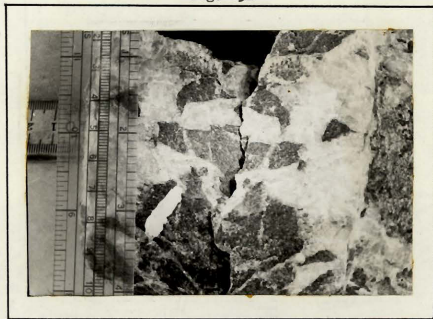
Photograph showing mirror sides of a split hand specimen. Angular unsupported fragments of "soft massive" peridotite in white glassy quartz
