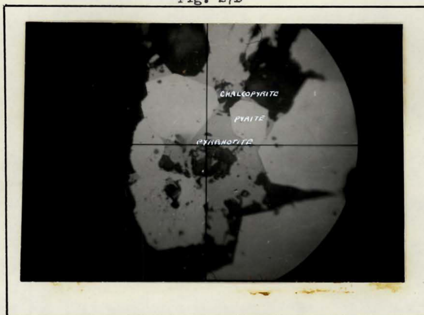
Relationships of Pyrite, Pyrrhotite, and Chalcopyrite (reflected light x 280)
