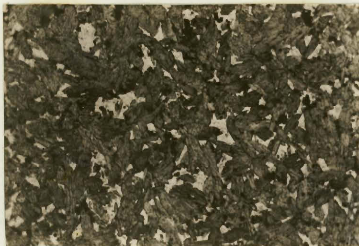
Fresh "diorite" in "hard massive" Peridotite at East Malartic (Ordinary light x 25)
