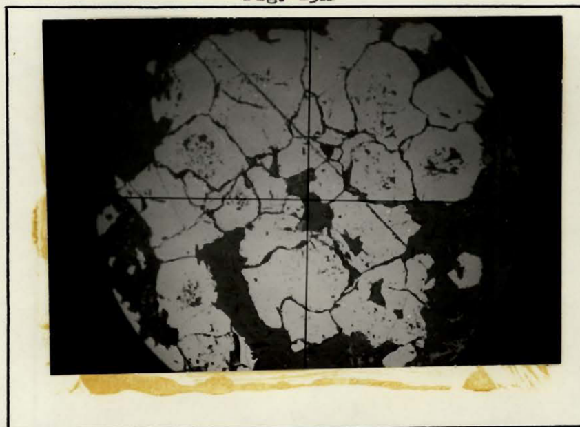
Cluster of pyrite crystals in ore "diorite" (reflected light x 70) showing silicate mineral nuclei. Note the general lack of fracturing of pyrite
