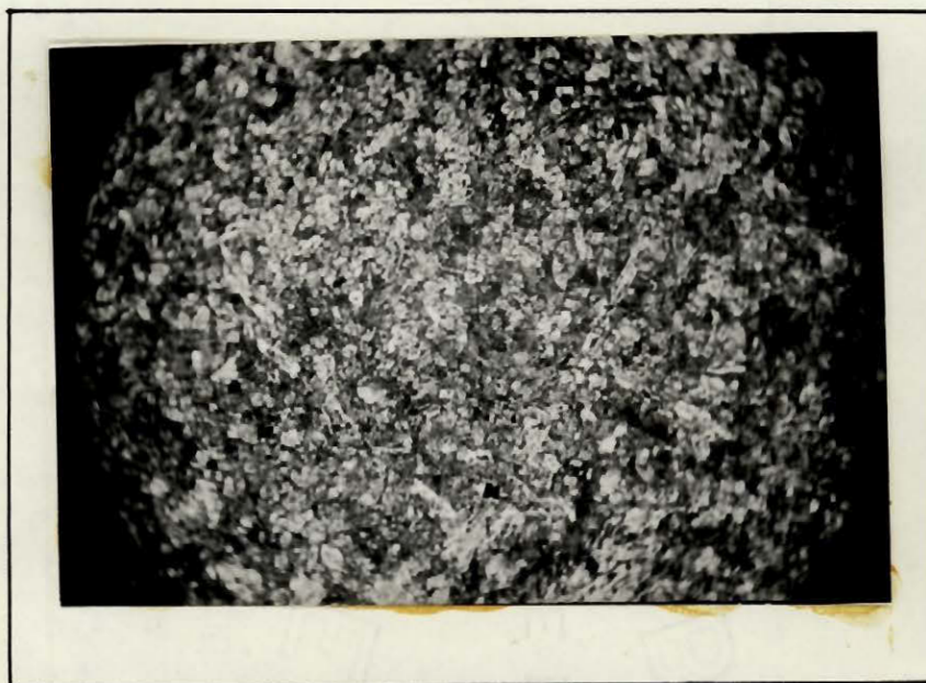
"Hard Massive" Peridotite (X nicols Mag. x 40) showing Granoblastic texture
