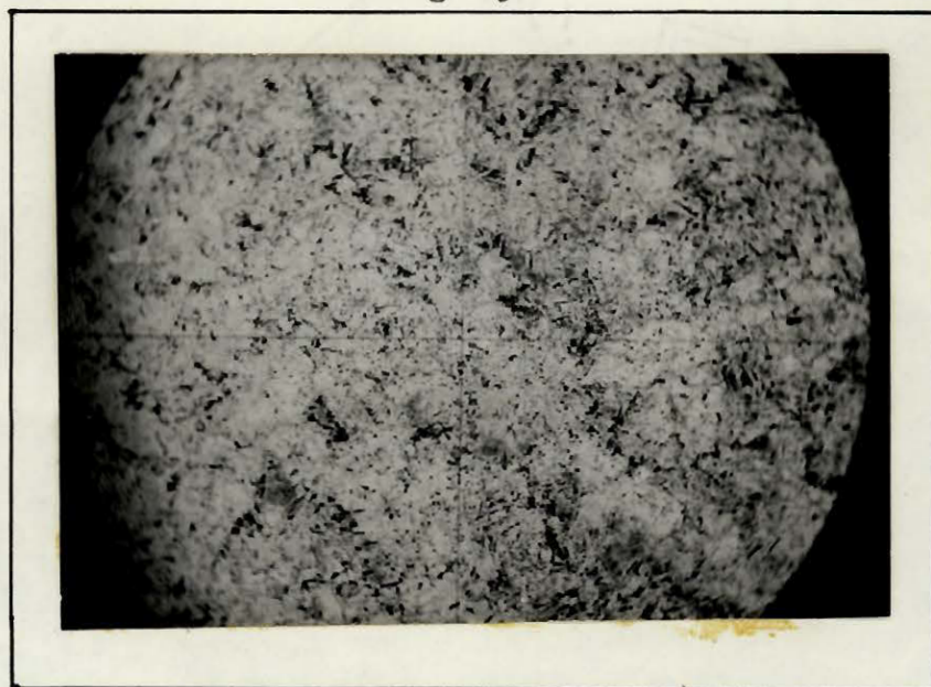
"Hard Massive" Peridotite (Ordinary light - Mag. x 40) showing finely dispersed magnetite
