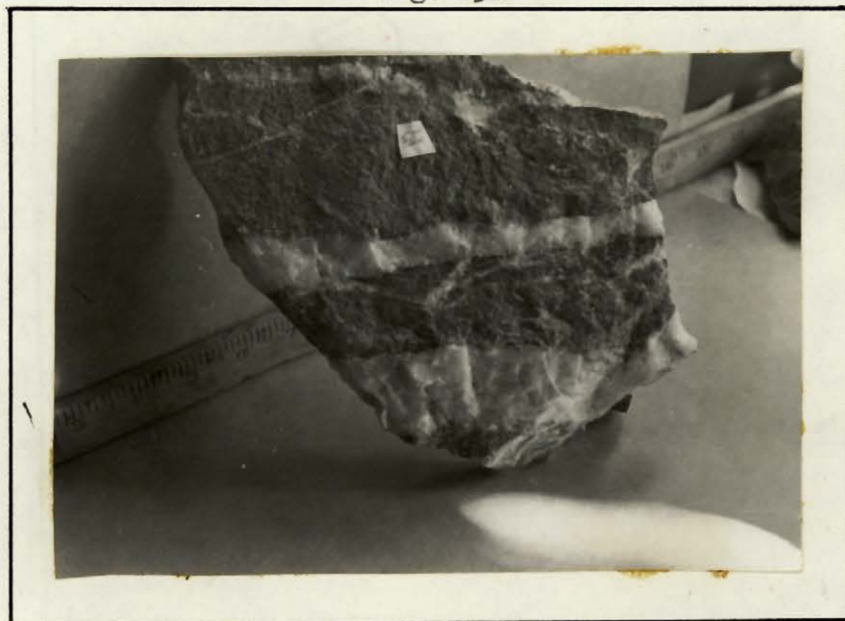
Photograph of hand specimen showing book structure in quartz veins in "diorite" Note: Triangular fragment of "diorite" at lower border of the center vein with no evidence of displacement
