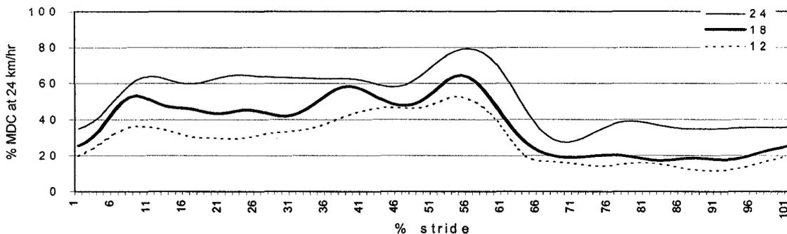
**FIGURE 9: M. BICEPS FEMORIS: GROUP AVERAGE EMG PATTERNS OF FORWARD SKATING AT THREE VELOCITIES; 12, 18, and 24km/hr**
