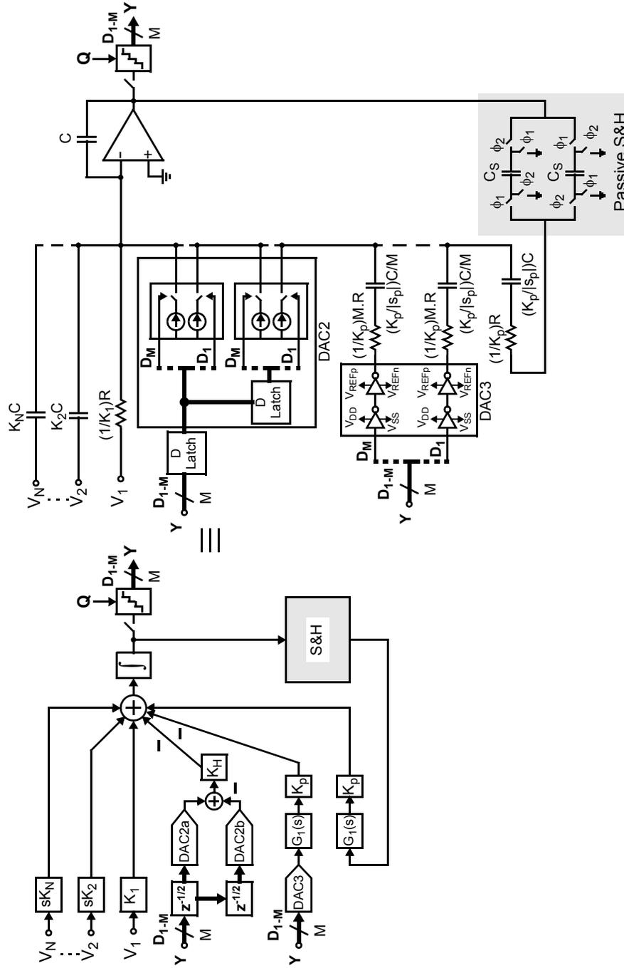
**Figure 3.3** Single-ended circuit implementation of the last integrator (Integ. 1) in Fig. 3.2. Here,  $C$  and  $R$  are unit-size capacitors and resistors;  $C_S$  is the sampling capacitor;  $V_{REFP}$  and  $V_{REFN}$  are the positive and negative reference voltages of the quantizer;  $M$  is the number of output thermometer digits (input threshold levels) of the quantizer.
