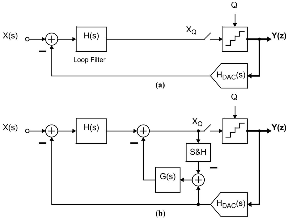
**Figure 1.1** Block diagram of (a) a classical CT  $\Delta\Sigma$  modulator; and (b) a CT  $\Delta\Sigma$  modulator with NTF enhancement.
