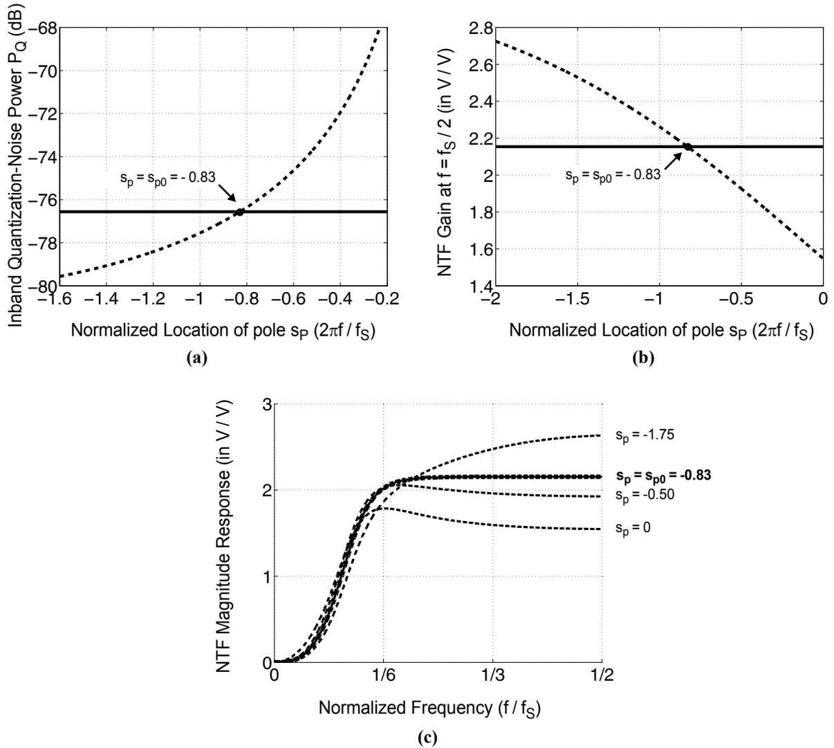
**Figure 2.3** Effect of the location of pole  $s_p f_S$  of the NTF-enhancement filter  $G_1(s)$  on: (a) the inband quantization-noise power  $P_Q$ ; (b) the NTF gain at  $f = f_S/2$  (i.e., at  $z = e^{j\pi}$ ); and (c) the magnitude response of the NTF for a  $\Delta\Sigma$  modulator with an *enhanced* 2<sup>nd</sup>-order Butterworth NTF (dashed lines - - -) versus a  $\Delta\Sigma$  modulator with a *classical* 3<sup>rd</sup>-order Butterworth NTF (solid lines —). OSR = 8.
