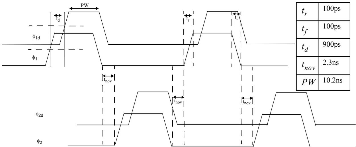
**Figure 5.10** Four phase non-overlapping clocking scheme for comparator in Fig. 5.9.
