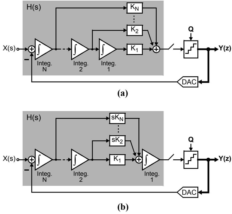
**Figure 3.1**  $N^{\text{th}}$ -order feedforward CT  $\Delta\Sigma$  modulator with: **(a)** classical feedforward compensation; **(b)** feedforward summation at the input of the last integrator. Here,  $\int \equiv 1/(sT_s)$ .
