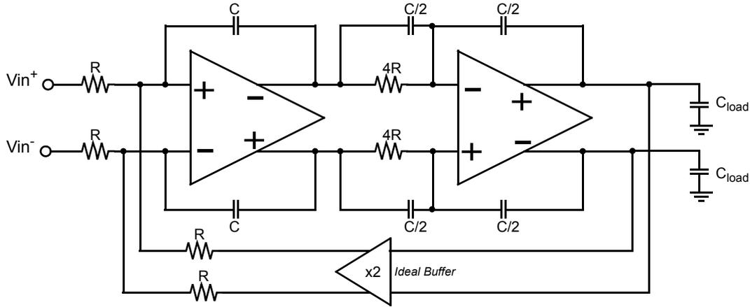
**Figure 5.18** Loop filter  $H(s)$  for the NTF-enhanced 2<sup>nd</sup>-order CT  $\Delta\Sigma$  modulator in Fig. 5.1, including output-level scaling.
