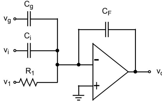
**Figure 4.3** Schematic of a single-ended CT integrator (in Fig. 3.3) with an integration path ( $R_1$ ),  $i$  feedforward summation paths ( $C_i$ ) and an NTF-enhancement feedback path ( $C_g$ ).
