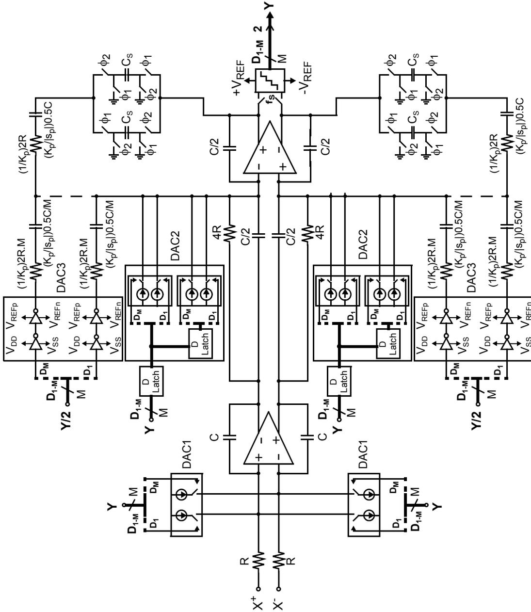
**Figure 5.5** Fully-differential circuit-level implementation of the NTF-enhanced 2<sup>nd</sup>-order feedforward CT  $\Delta\Sigma$  Modulator in Fig. 5.1 with output-level scaling ( $K_a = 0.5$ ,  $K_d = 2$ ). Here  $C$  and  $R$  are unit capacitors and unit resistors respectively such that  $f_S = 1/RC$  and  $C_S$  is the sampling capacitor.  $V_{REFp}$  and  $V_{REFn}$  are the quantizer positive and negative reference voltages respectively and  $M$  is the number of quantizer levels.
