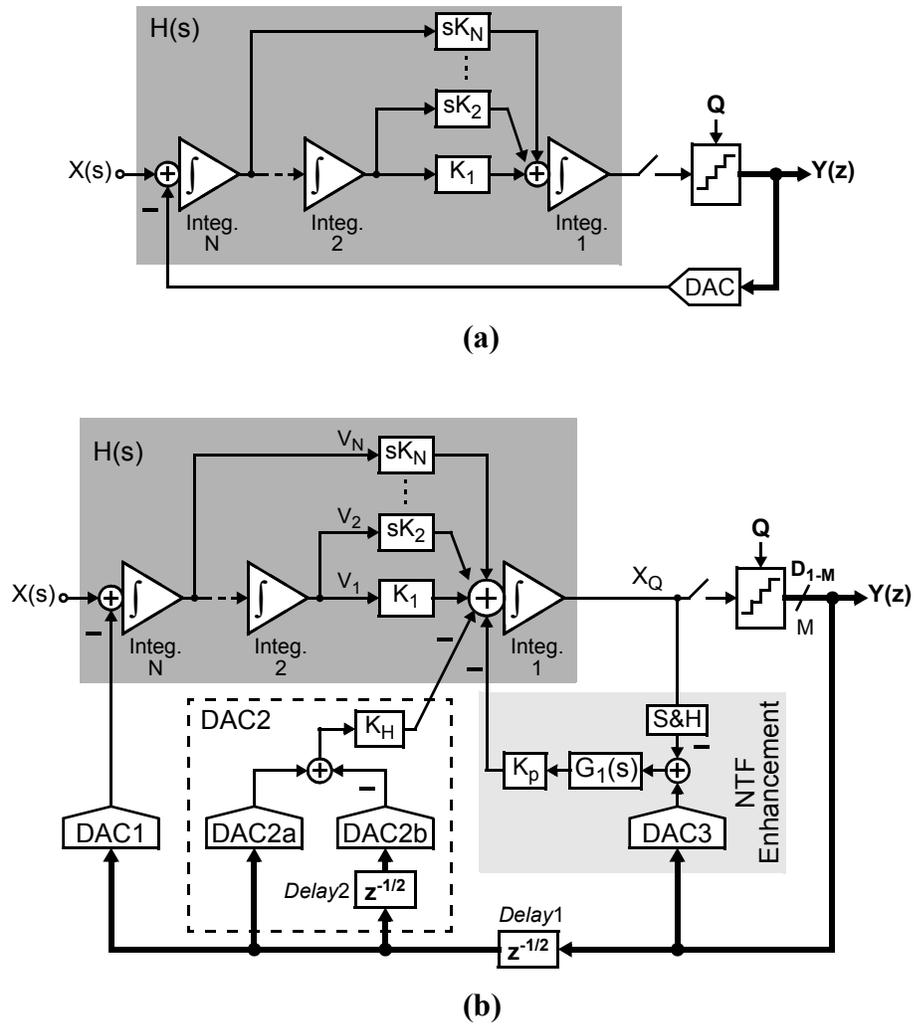
**Figure 4.5**  $N^{\text{th}}$ -order feedforward CT  $\Delta\Sigma$  modulator with: (a) classical feedforward architecture. (b) proposed architecture with NTF enhancement and excess-loop-delay compensation (using feedback path  $K_H$  through DAC2). Here,  $\int \equiv 1/(sT_S)$ .
