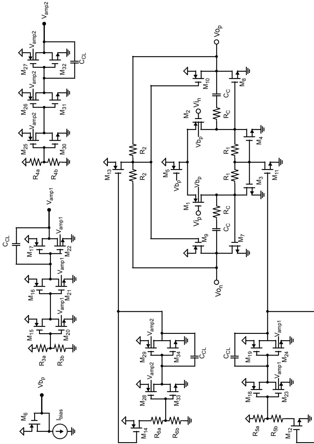
**Figure 5.7** Complete circuit-level schematic for the fully-differential 2-stage Opamp with lead compensation [Johns 97]
