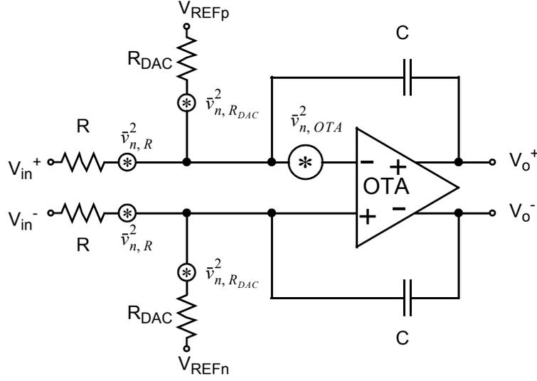
**Figure 4.2** Schematic of a fully differential active RC-integrator with thermal noise sources.
