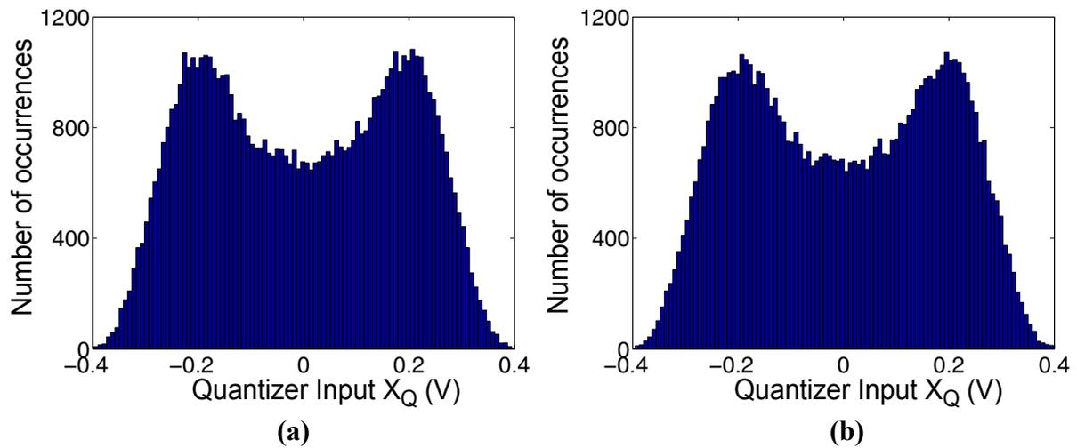
**Figure 5.3** Histogram of the quantizer input signal level  $X_Q$  for the NTF-enhanced 2<sup>nd</sup>-order CT  $\Delta\Sigma$  modulator in Fig. 5.1: (a) with output-level scaling ( $K_a = 0.5, K_d = 2$ ); and (b) without output-level scaling ( $K_a = 1, K_d = 1$ ). ( $V_{REF} = v_{o, sat} = 0.7$  V, OSR = 20,  $V_{in} = -3.1$  dBFS).
