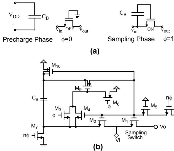
**Figure 5.14** Bootstrapped switch design for the comparator in Fig. 5.9: **(a)** Conceptual diagram depicting its operation; **(b)** Circuit-level implementation [Dessouky, JSSCC01].
