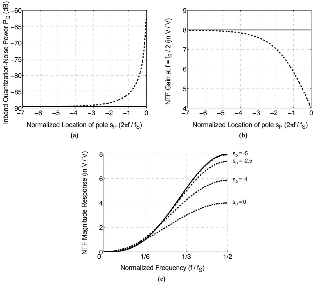
**Figure 2.2** Effect of the location of pole  $s_p f_S$  of the NTF-enhancement filter  $G_1(s)$  on: (a) the inband quantization-noise power  $P_Q$ ; (b) the NTF gain at  $f = f_S/2$  (i.e., at  $z = e^{j\pi}$ ); and (c) the magnitude response of the NTF for a  $\Delta\Sigma$  modulator with an *enhanced* 2<sup>nd</sup>-order FIR NTF (dashed lines ---) versus a  $\Delta\Sigma$  modulator with a *classical* 3<sup>rd</sup>-order FIR NTF (solid lines —). OSR = 8.
