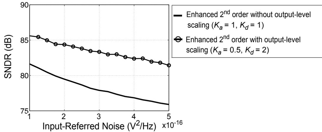
**Figure 5.2** Effect of thermal noise on SNR performance of the NTF-enhanced 2<sup>nd</sup>-order CT  $\Delta\Sigma$  modulator in Fig. 5.1. ( $V_{REF} = v_{o, sat} = 0.7$  V, OSR = 20,  $V_{in} = -3.1$  dBFS).
