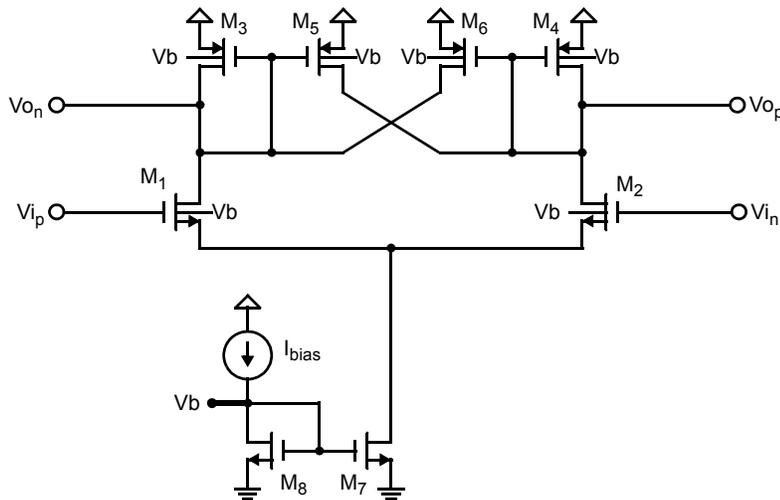
**Figure 5.11** Preamplifier circuit for the comparator in Fig. 5.9 [Gregorian 99, Fig. 5.16].
