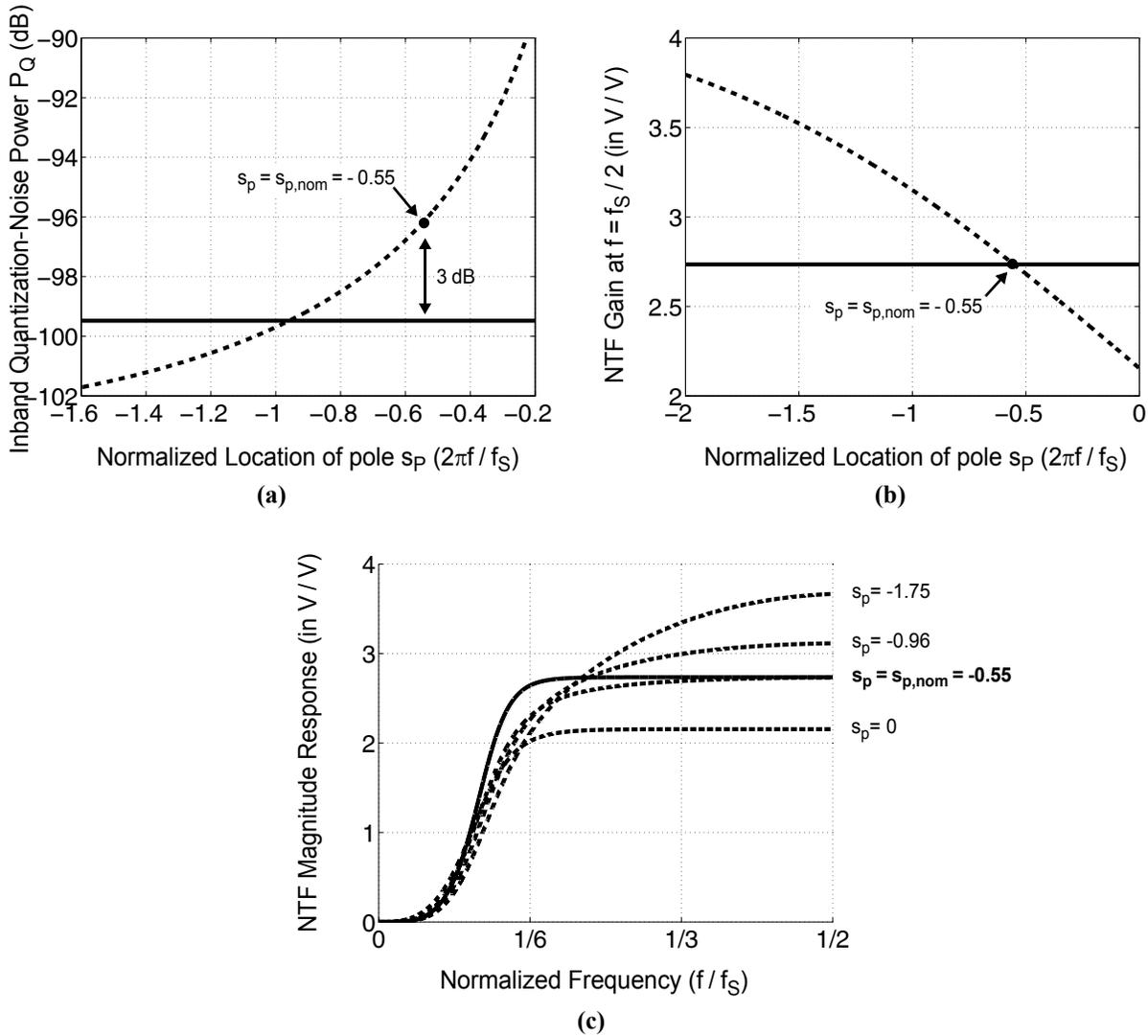
**Figure 2.4** Effect of the location of pole  $s_p f_S$  of the NTF-enhancement filter  $G_1(s)$  on: (a) the inband quantization-noise power  $P_Q$ ; (b) the NTF gain at  $f = f_S / 2$  (i.e., at  $z = e^{j\pi}$ ); and (c) the magnitude response of the NTF for a  $\Delta\Sigma$  modulator with an *enhanced* 3<sup>rd</sup>-order Butterworth NTF (dashed lines - - -) versus a  $\Delta\Sigma$  modulator with an *classical* 4<sup>th</sup>-order Butterworth NTF (solid lines —). OSR = 8.
