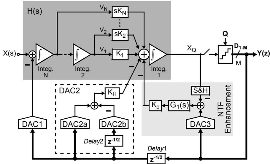
**Figure 3.2** Proposed  $N^{\text{th}}$ -order feedforward CT  $\Delta\Sigma$  modulator with NTF enhancement and excess-loop-delay compensation (using feedback path  $K_H$  through DAC2). Here,  $\int \equiv 1/(sT_S)$ .
