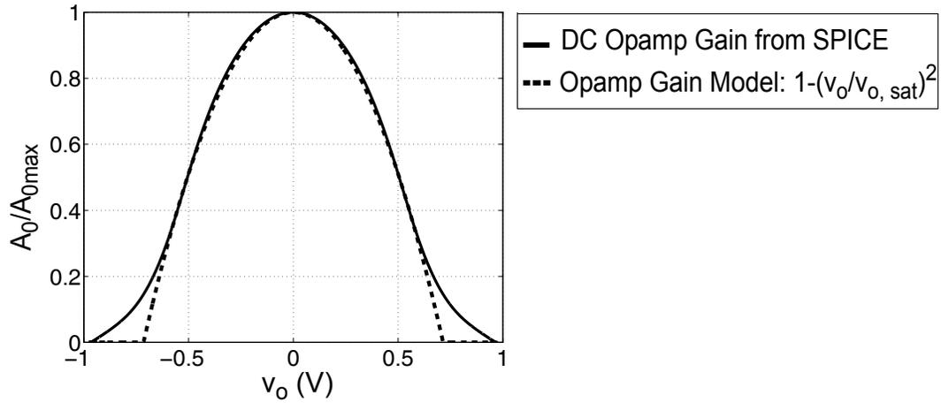
**Figure 5.8** Opamp nonlinear dc gain determined from SPICE and from the gain model in (4.15).  $A_0$  is the dc opamp gain,  $v_o$  is the output voltage and  $v_{o, sat}$  is the opamp output saturation voltage.  $v_{o, sat} = 0.7$  V.
