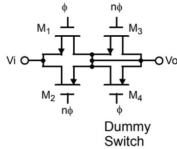
**Figure 5.15** Transmission-gate switch for the comparator in Fig. 5.9, including dummy structure to reduce charge injection errors.
