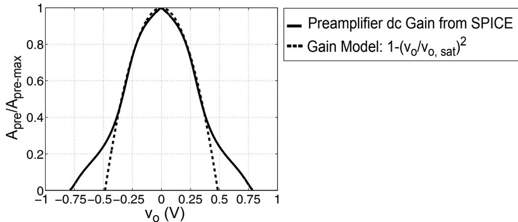
**Figure 5.12** Nonlinear dc gain  $A_{pre}$  for the preamplifier in Fig. 5.11, determined from SPICE.  $v_o$  is the output voltage and  $v_{o, sat}$  is the output saturation voltage.
