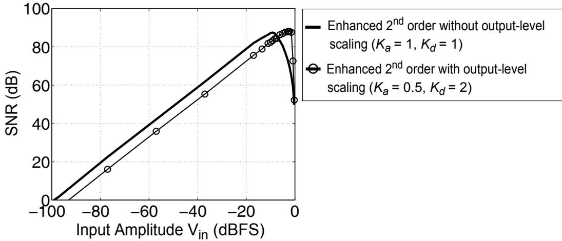
**Figure 5.4** Effect of output-level scaling on SNR performance of the proposed NTF-enhanced 2<sup>nd</sup>-order CT  $\Delta\Sigma$  modulator in Fig. 5.1 ( $V_{REF} = v_{o, sat} = 0.7$  V,  $OSR = 20$ ,  $V_{in} = -3.1$  dBFS,  $DR = 90$ dBFS).
