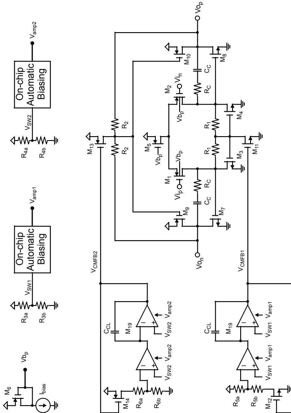
**Figure 5.6** Fully-differential 2-stage Opamp with lead compensation [Johns 97]. The conceptual schematic for the CMFB circuit is shown here [Chatterjee, JSSC05].
