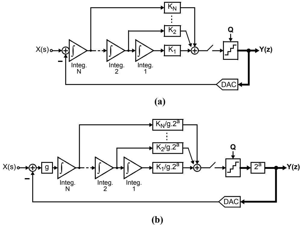
**Figure 4.1**  $N^{\text{th}}$ -order feedforward CT  $\Delta\Sigma$  modulator with: **(a)** classical architecture; **(b)** output voltage-level scaling. Here,  $\int \equiv 1/(sT_S)$ ,  $g$  is a scaling coefficient and  $a$  is an integer.
