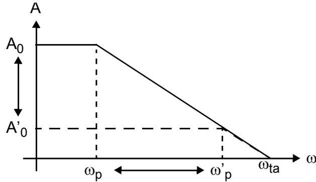
**Figure 4.4** Effect of nonlinear variations in opamp dc gain on its frequency response.
