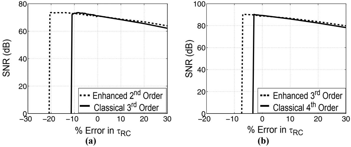
**Figure 4.7** Effect of errors in integrator  $RC$  time constants ( $\tau_{RC}$ ) on SNR performance of the NTF-enhanced  $N^{\text{th}}$ -order and classical  $(N+1)^{\text{th}}$ -order feedforward CT  $\Delta\Sigma$  modulators, for: **(a)**  $N = 2$ ; and **(b)**  $N = 3$ . Here,  $OSR = 12$ ,  $V_{in} = -6.2$  dBFS and all integrators have a large  $K_{GBW} = 5$ . Integ. 1 has a constant dc gain  $A_0 = 50$  dB and all previous integrators have a constant dc gain  $A_0 = 45$  dB.
