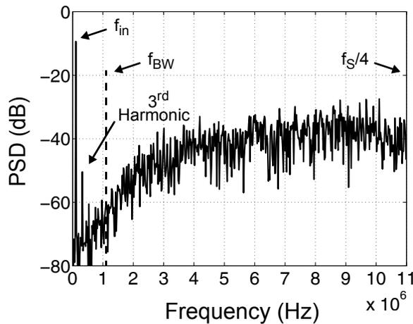
**Figure 5.20** Output power spectral density (PSD) for the NTF-enhanced CT  $\Delta\Sigma$  modulator in Fig. 5.19.
