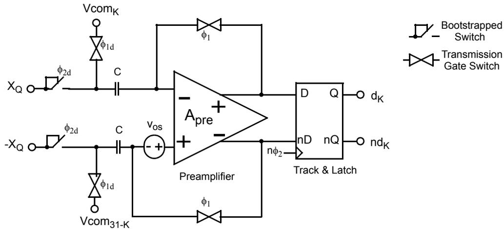
**Figure 5.9** Comparator unit cell with input-offset storage, preamplifier and track-and-latch [Gregorian 99].
