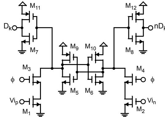
**Figure 5.16** Ratioed CMOS Latch for the comparator in Fig. 5.9 [Rabaey 03, Fig. 7-21].
