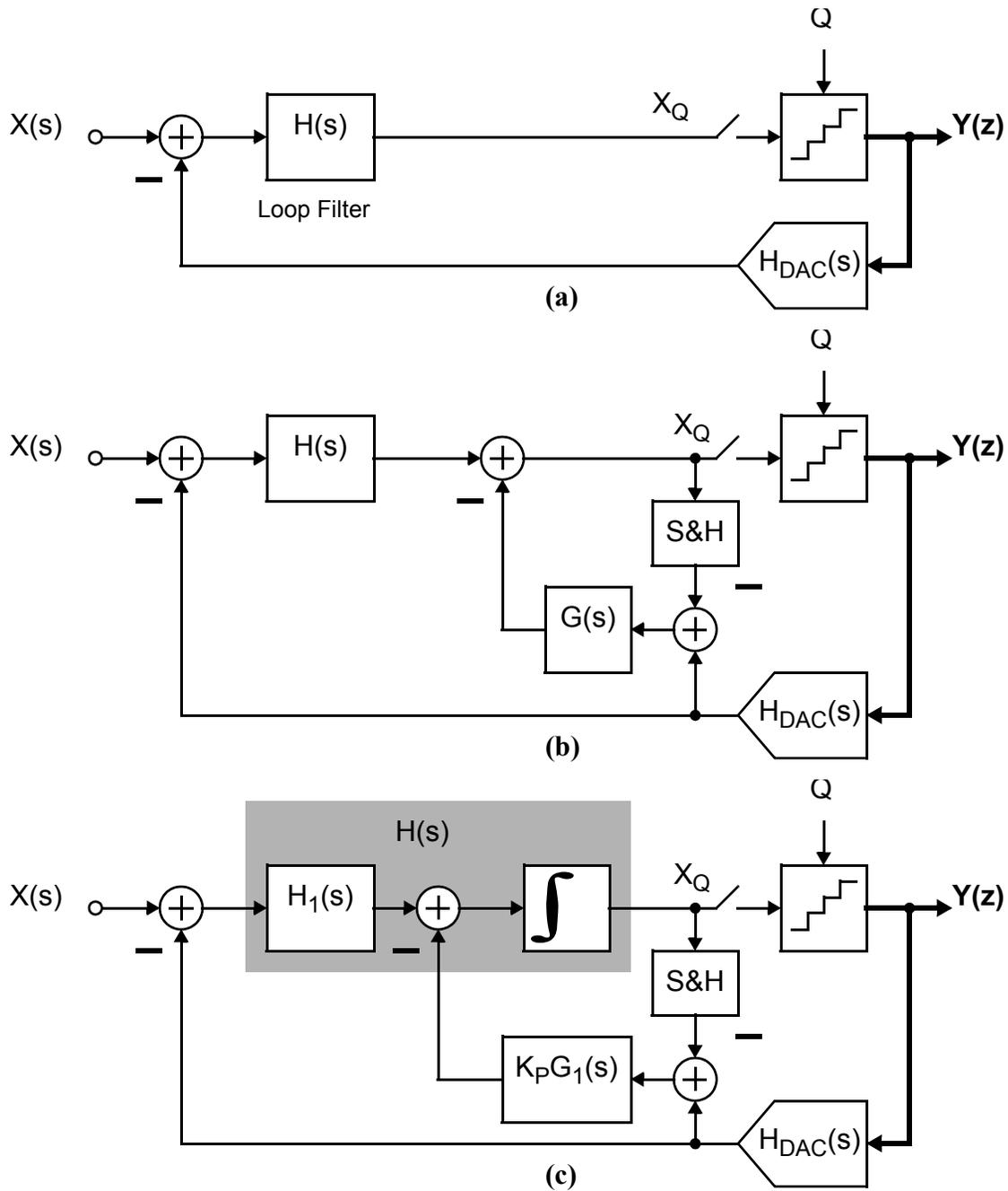
**Figure 2.1** Block diagram of: (a) a classical CT  $\Delta\Sigma$  modulator; (b) a CT  $\Delta\Sigma$  modulator with NTF enhancement; and (c) the proposed simplified realization of the  $\Delta\Sigma$  modulator in (b). Here,  $\int \equiv 1/(sT_S)$ .
