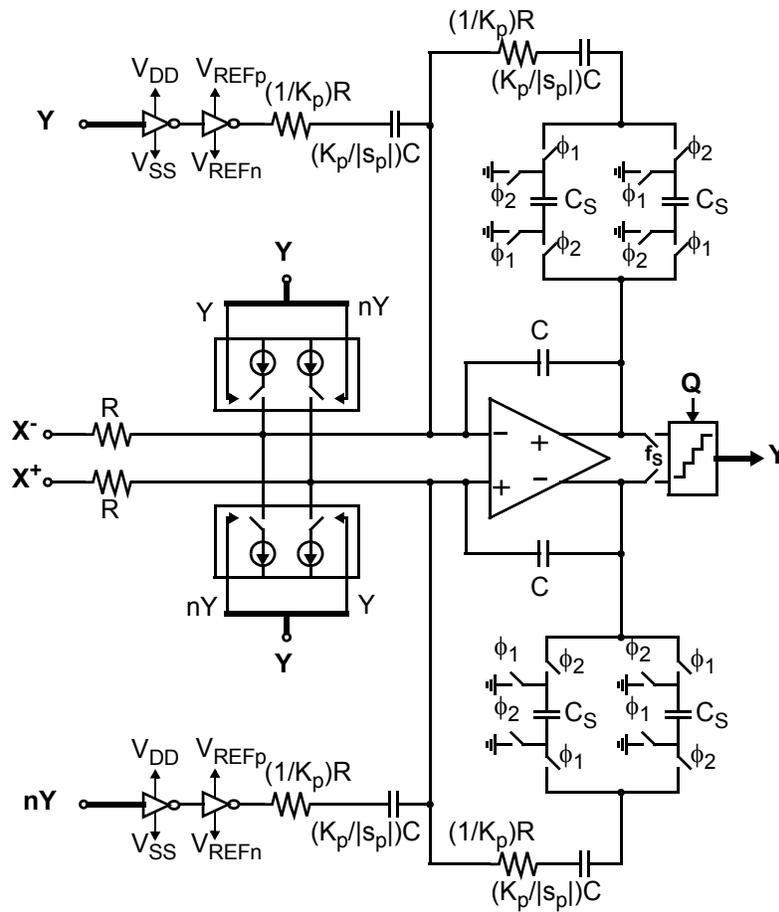
**Figure 5.19** Circuit implementation of NTF-enhanced 1<sup>st</sup>-order CT  $\Delta\Sigma$  modulator with 1-bit quantizer and passive S&H, used to verify the functionality of the NTF-enhancement filter  $G_1(s)$  in Fig. 5.1. Here, excess-loop-delay is not included.
