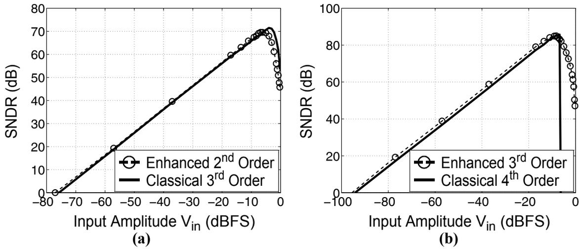
**Figure 4.8** Effect of input-signal amplitude  $V_{in}$  on SNDR performance of the NTF-enhanced  $N^{\text{th}}$ -order and classical  $(N+1)^{\text{th}}$ -order feedforward CT  $\Delta\Sigma$  modulators, for: **(a)**  $N = 2$ , Integ. 1 has  $A_{0\text{max}} = 50$  dB and  $K_{GBW} = 3$ ; and **(b)**  $N = 3$ , Integ. 1 has  $A_{0\text{max}} = 50$  dB and  $K_{GBW} = 5$ . Here,  $\text{OSR} = 12$  and all previous integrators have  $A_{0\text{max}} = 45$  dB and  $K_{GBW} = 1$ .
