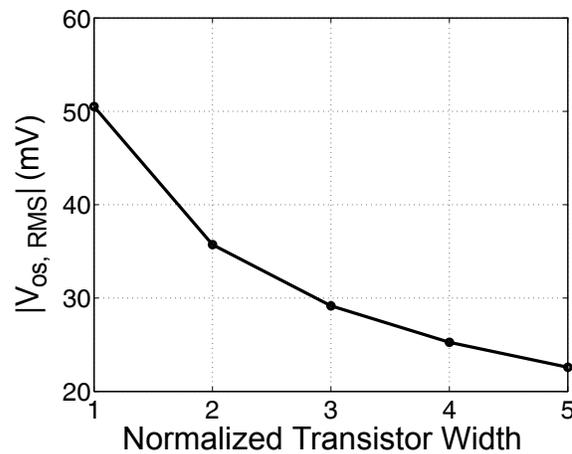
**Figure 5.13** Absolute input-referred RMS offset voltage  $v_{os, RMS}$  for the preamplifier in Fig. 5.11. A normalized transistor width of 1 corresponds to a min-sized transistor. The monte-carlo simulations performed in SPICE included mismatch and process variations in the transistor widths as well as their threshold voltages.
