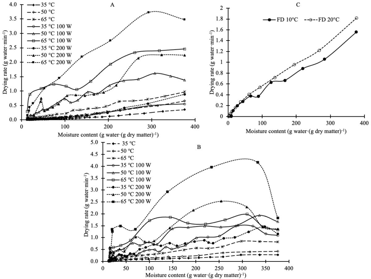
Figure 5.3. Drying rate curves of (A) untreated, (B) pre-frozen at  $-80^{\circ}\text{C}$ , and (C) freeze dried hops.
