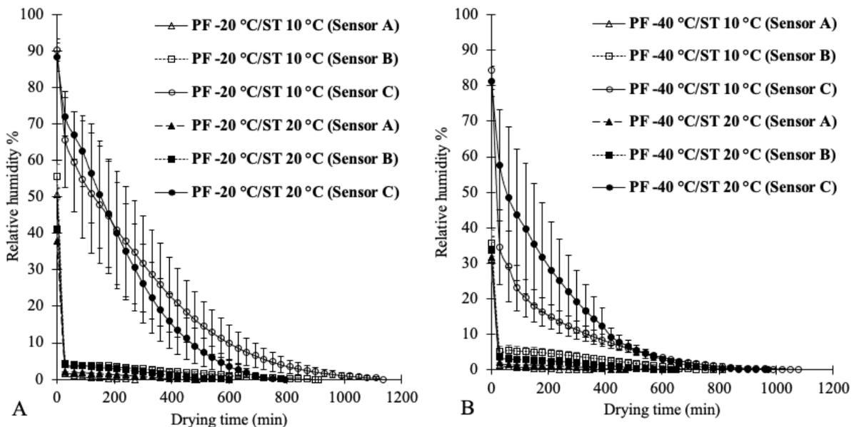
Figure 6.4. Relative humidity for Qrazy Train subjected to different pre-freezing temperatures (PF) and freeze-drying shelf temperatures (ST).
