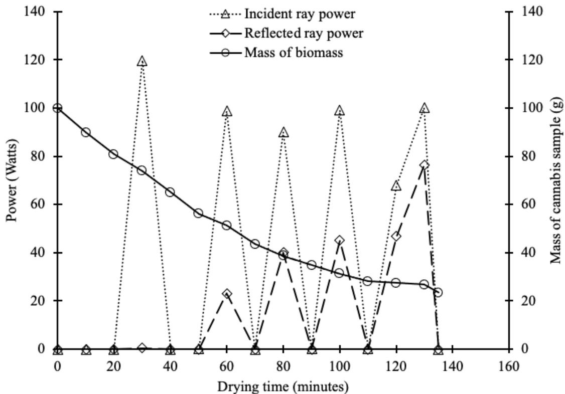
Figure 13.4. Changes in the mass of samples, incident power and reflected power during microwave drying.
