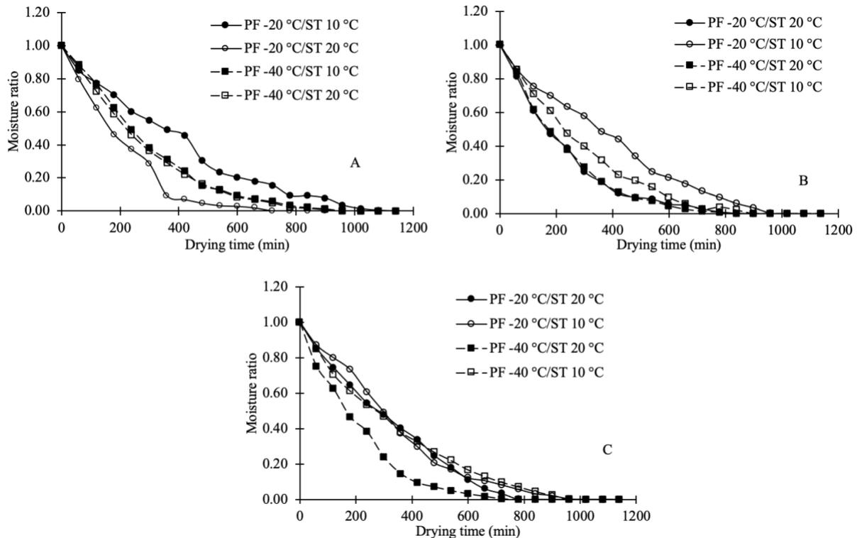
Figure 6.8. Moisture ratio curves of for Qrazy Train (A), Qrazy Apple (B), and Qrazy Angel (C) submitted to different pre-freezing (PF) and freeze-drying shelf temperatures (ST).
