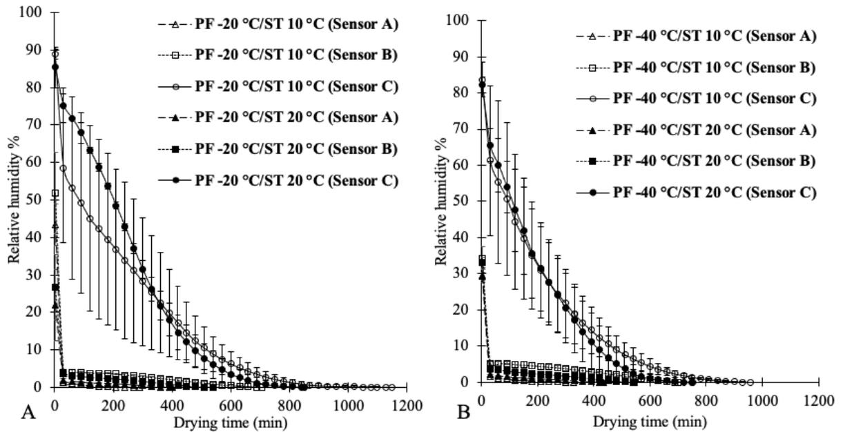
Figure 6.6. Relative humidity values for Qrazy Angel subjected to different pre-freezing temperatures (PF) and freeze-drying shelf temperatures (ST).
