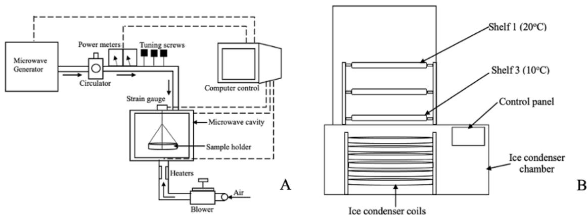
Figure 5.1. Schematic diagram of the (A) microwave-assisted hot air dryer and (B) vacuum freeze dryer.
