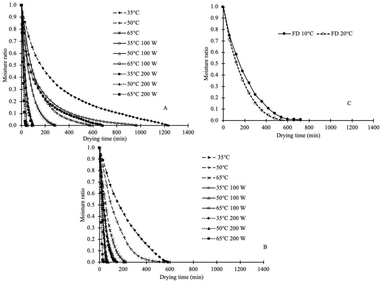
Figure 5.2. Moisture ratio curves of (A) untreated, (B) pre-frozen at -80°C, and (C) freeze dried hops.
