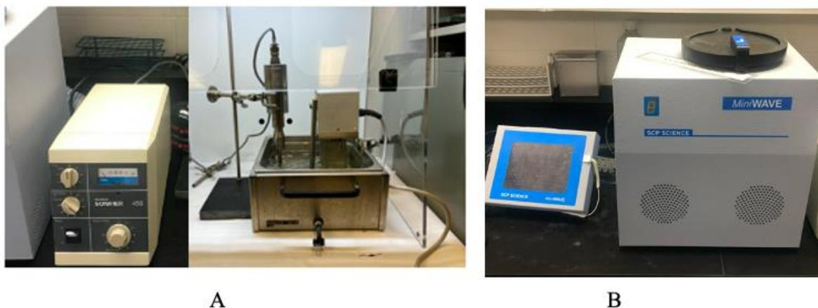
Figure 11.1. Branson Sonifier 450 ultrasound (A) and mini-wave microwave (B) extraction systems used for the study.
