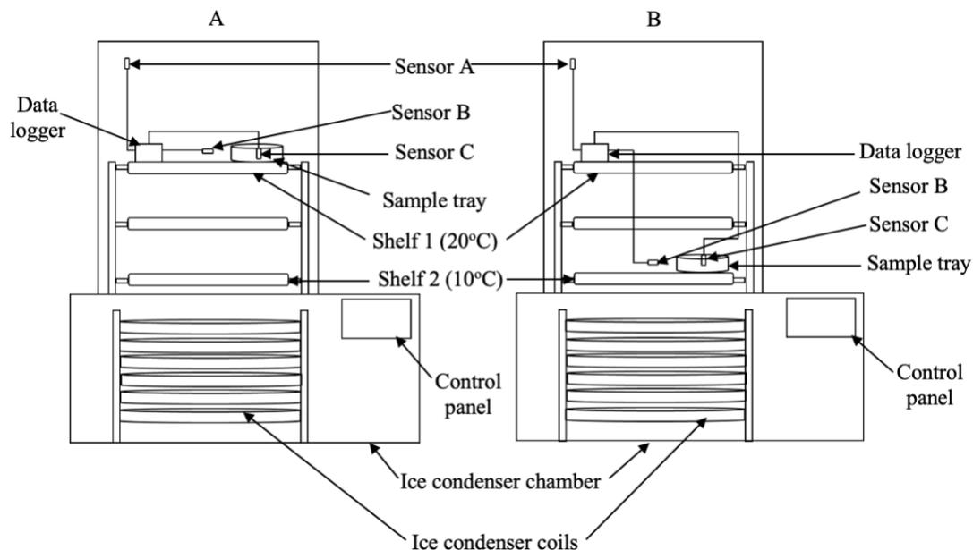
Figure 6.1. Sensor location and pre-frozen cannabis samples placed on (A) shelf 1 (top) and (B) shelf 2 (bottom) for the freeze-drying experiment.
