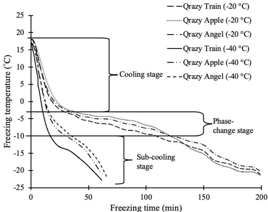
Figure 6.2. Pre-freezing curves for cannabis accessions submitted to different pre-freezing temperatures.
