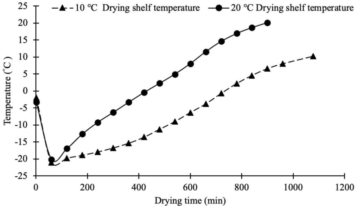
Figure 6.7. Comparison of freeze-drying curves of Qrazy Train pre-frozen at -20°C at different shelf temperatures.
