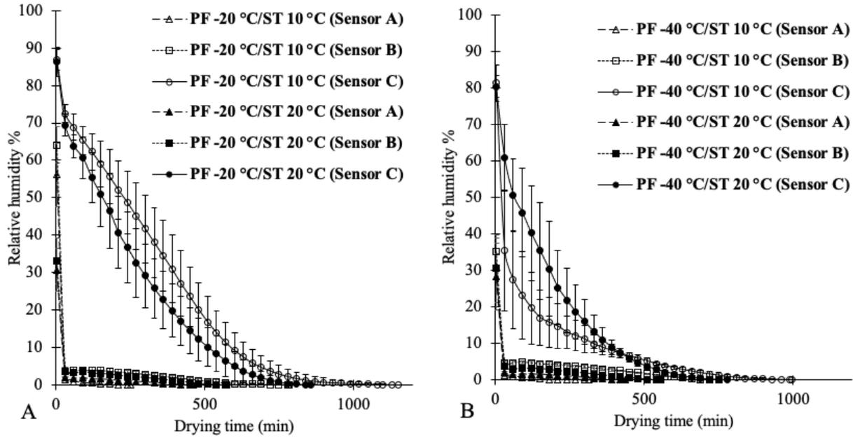
Figure 6.5. Relative humidity for Qrazy Apple subjected to different pre-freezing temperatures (PF) and freeze-drying shelf temperatures (ST).
