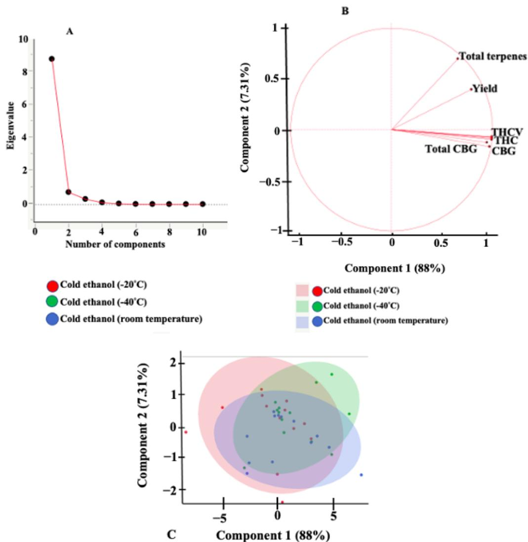
Figure 10.3. Scree (A), loadings (B), and scatter (C) plots for cold ethanol extraction of cannabis at  $-20^{\circ}\text{C}$ ,  $-40^{\circ}\text{C}$ , and room temperature.
