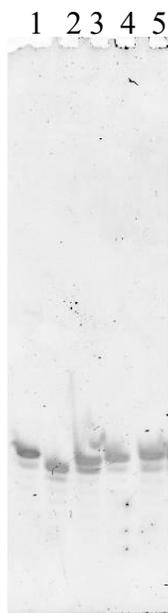
**Figure 5.14.** 15 % PAGE denaturing conditions, **AT-Ant**, **AT**, **AT-Bal**, **AT-His**, **AT-Trp**. Lanes 1 to 5: Crude mixtures from synthesis of **AT-Ant**, **AT**, **AT-Bal**, **AT-His**, **AT-Trp**. **Bal** is found to have lower attachment yields in this case because it is located at the 5' end. These strands were made and HPLC-purified in order to characterize them by LC-MS.
