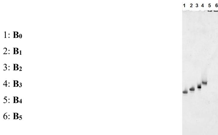
**Figure 2.21.** 15 % denaturing PAGE analysis of “DNA-Teflon” oligomers. The DNA is the AT sequence and the length of the PFC tail vary from 0 to 5 PFC units ( $B_n$  polymers). From  $n=4$ , self-assembly occurs and the material does not seem able to penetrate in the gel (non-penetrating band).
