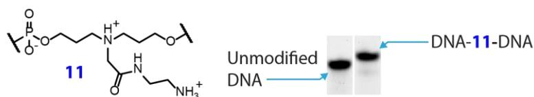
**Figure 4.6.** Attachment of amine-functionalized containing monomer in a DNA 21mer. 15 % PAGE in denaturing conditions. Yields were found to be over 94 % by gel image analysis.
