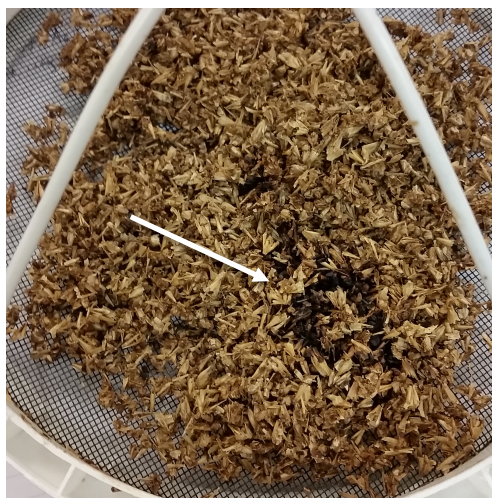
Figure 18. Burned BSG. Isolated burned grains after drying treatment.
