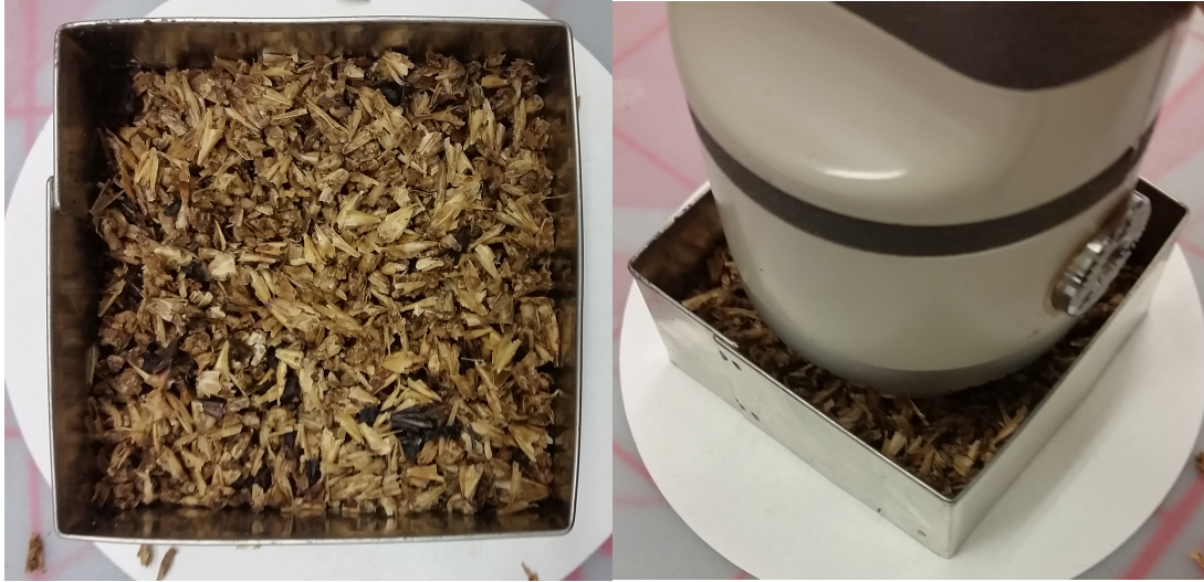
Figure 11. Grain color determination. The CIE color method was used to determine L^*a^*b^* color coordinates.
