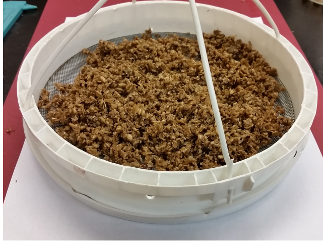
Figure 7. Dryer sample tray with brewers' spent grain sample.
