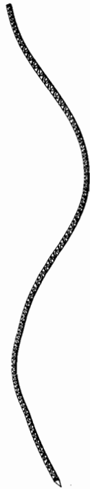
Fig. 4.4. Four lowest flexural mode shapes of the 198-m tower
