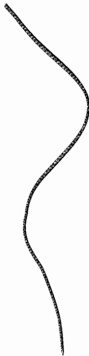
Fig. 4.6. Four lowest flexural mode shapes of the 213-m tower
