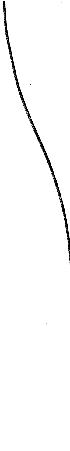
Fig. 5.33. First flexural natural mode shape of mast in the 607-m tower ( T = 4.27 s)
