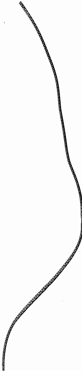
Fig. 5.28. First flexural natural mode shape of mast in the 342-m tower ( T = 2.10 s)
