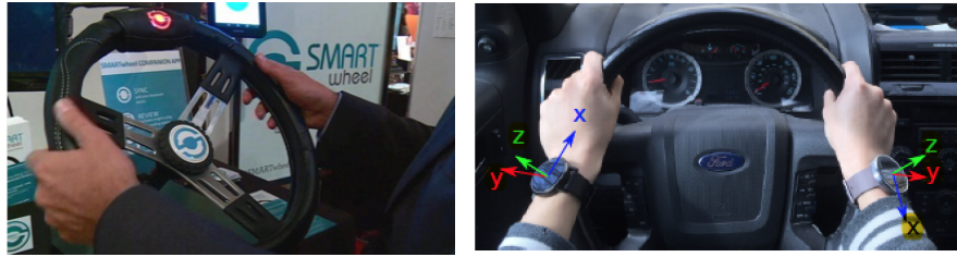
Figure 4.1 Existing work for detecting hands on or off the steering wheel. (1) SMARTwheel system [1] and (2) SafeWatch [2]
