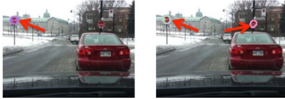
Figure 3.9 An Example of Adaptive Color Filtering. The stop sign detection failed without weather-adaptive color range (left). With the aid of adaptive range selection, SafeCam is able to detect stop signs on both sides of the road (right).
