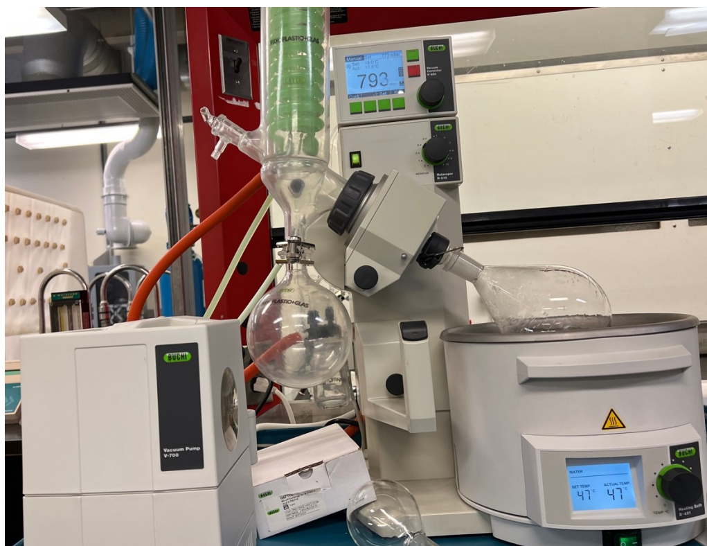
Figure 10 Overview of the rotary evaporation system
