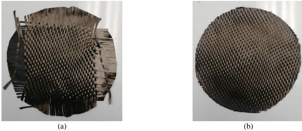
Figure 6: (a) Examples of cut ply without binder showing signs of frayed edges (b) and fabric with binder showing no signs of frayed edges.
