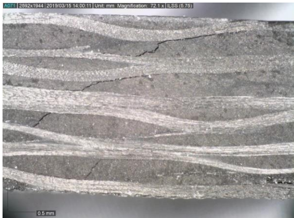
Figure 47: Typical interlaminar shear failure mode observed with SB_REF and SB_ME samples
