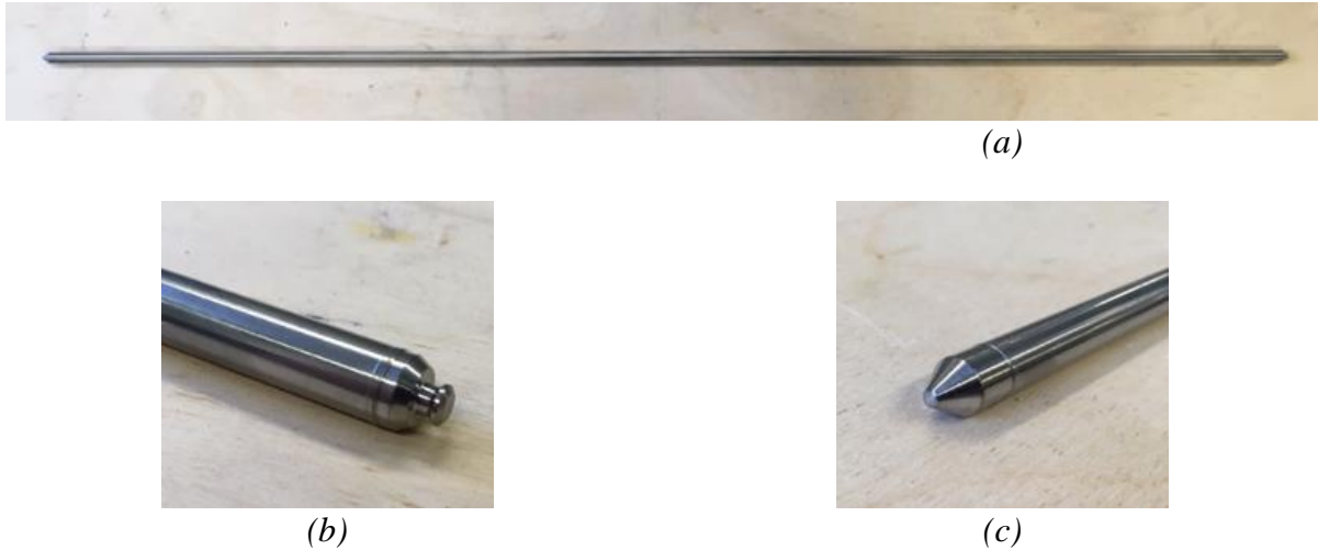
Fig. 5-1: Zirconium fuel rod under test, (a). Clamping end (b); insertion end (c).
